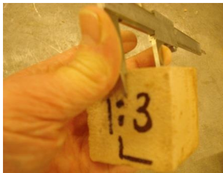
Figure 5: Measurement of cube dimensions using vernier callipers
