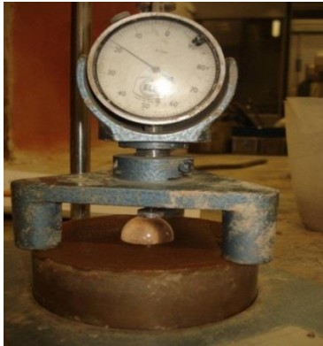
Figure 1: Dropping ball equipment for measuring workability
