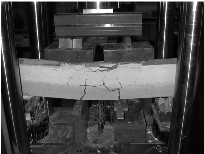
Figure 3. Flexural testing of deteriorated reinforced concrete beams.
