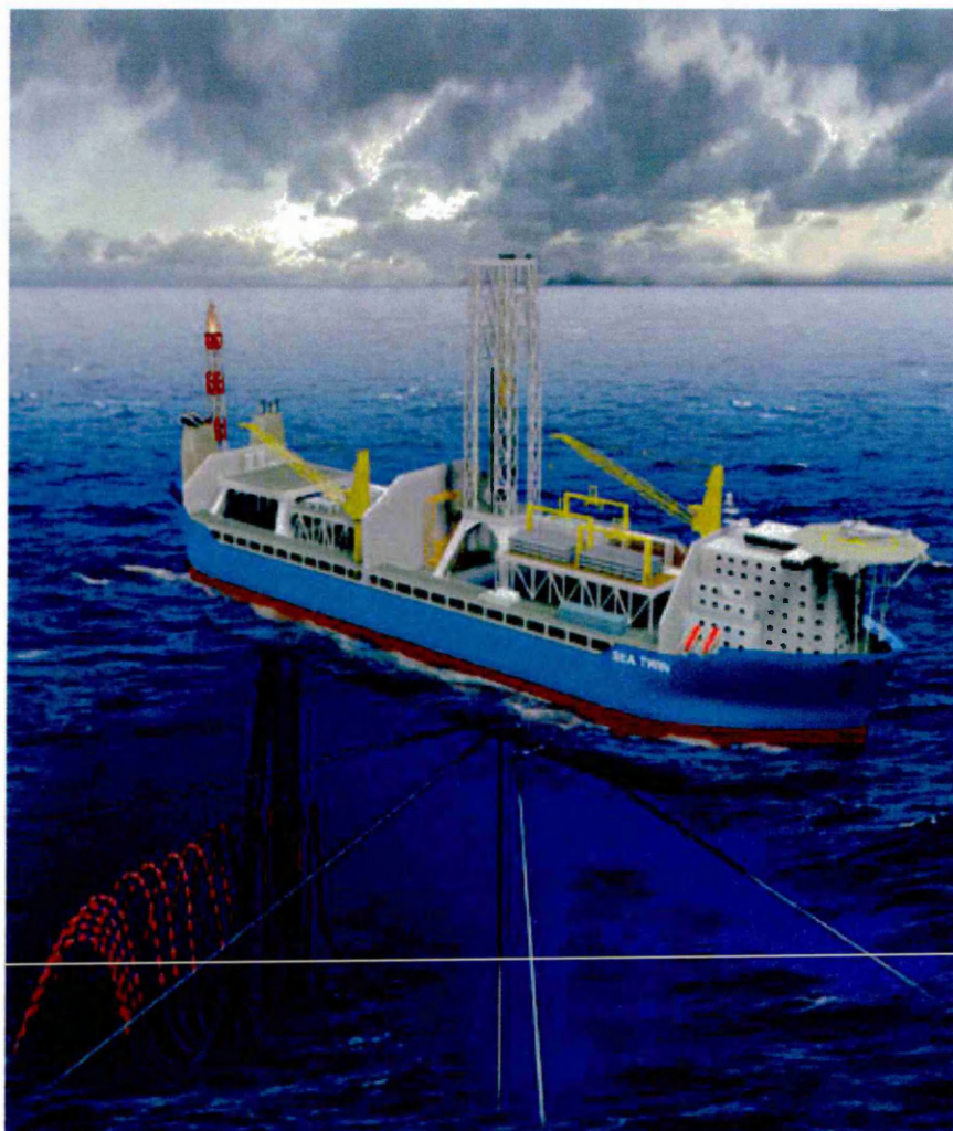
FIGURE D.3: Risers are connected to typical FPSO as wave catenary
