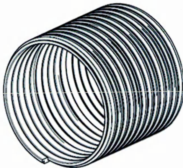
FIGURE 3.3: Pressure Armour Layer
