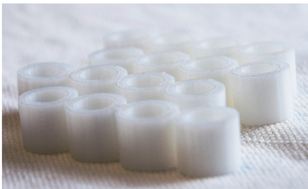
Figure 5. 3D FDM-printed modular tubes.
