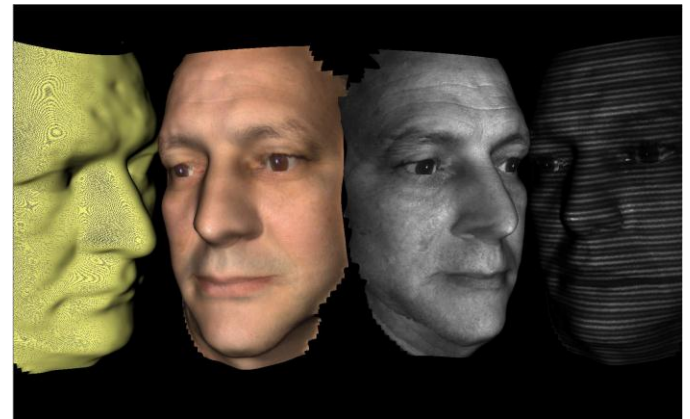
Figure 6. Triangulated mesh (left), with color and black and white texture mapping (centre) and with original stripe pattern (right)
