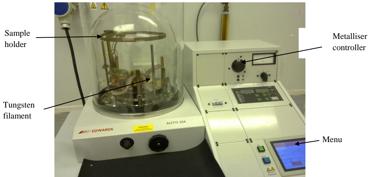
Figure 3.1: A photograph of an EDWARD metalliser.
