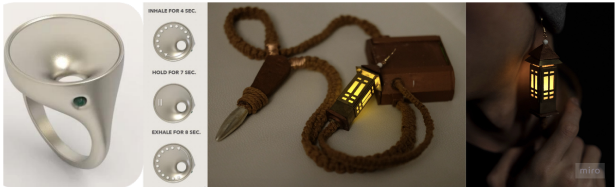
Figure 6 (left to right) a) Interlude . A visual representation of the ring and its functionality, b) Wabi-sabi : A set consisting of a digital earring and necklace, showing the wearer engaging with the earring.
