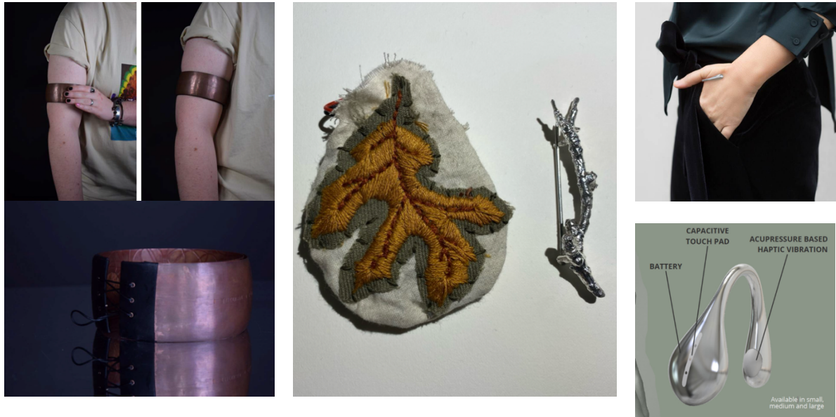
Figure 7 (left to right) a) Amulet for Anxiety : (top) The wearer touches the piece to activate the vibration. (bottom) Detail of the leather section that can be manually tightened. middle b) Nature : Detail of the embroidered bag that houses the electronics and the silver twig-shaped brooch. c) Alleviate : (top) Worn between the thumb and index finger, (bottom) showing a visual description of the electronic components.
