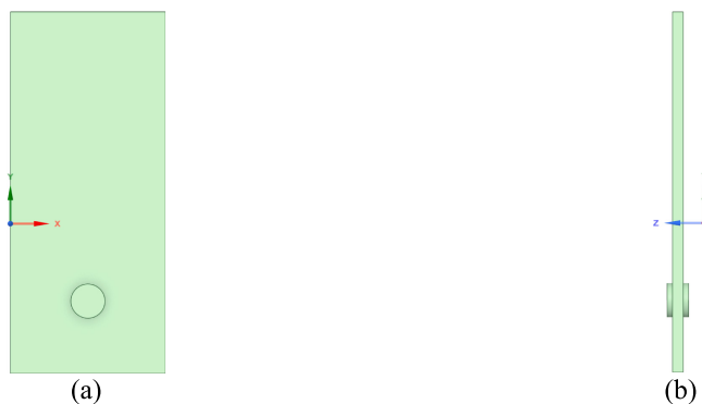
FIGURE 8 | Simplified model showing a single inner plate with a cylindrical bolt shank inserted through the hole: (a) front view and (b) side view. [Colour figure can be viewed at wileyonlinelibrary.com ]
