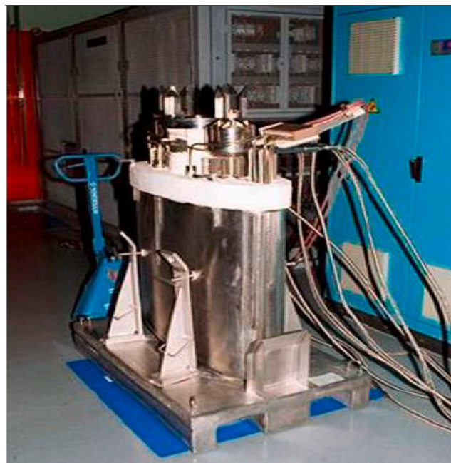
Fig. 6. Photograph of La Hague hot-walled induction melter (HWIM). Reprinted from Vienna et al. [10] with permission from The American Ceramic Society and Wiley Periodicals, Inc.
