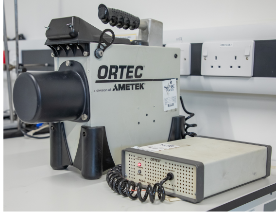
Figure 4.2: A Photograph of the Trans-SPEC detector in the RADLab at the UKAEA, with the external power unit attached
