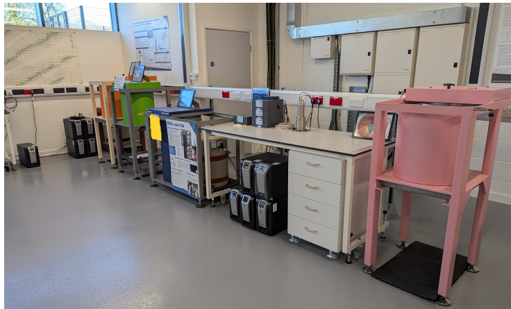
Figure 1.2: The RADLab, at the UKAEA's Culham Campus. The photograph shows a corner of the RADLab, where static HPGe detectors are housed within lead castles (orange, green, blue, and pink)
