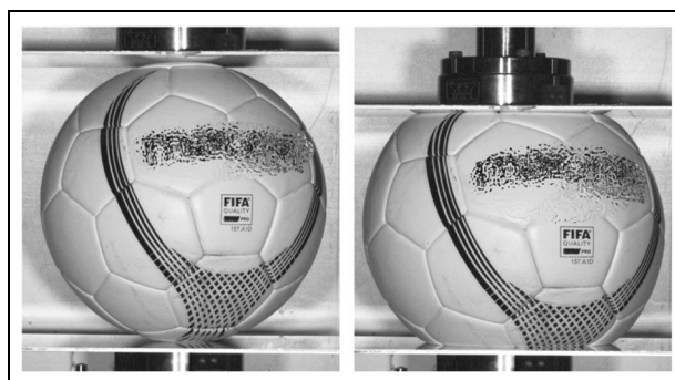
Figure 1. Images of the quasi-static compression test of a football: (a) The upper plate moves at a slow, controlled rate with uniform force application to compress a football from its uncompressed state to (b) a deflection of 45 mm.
