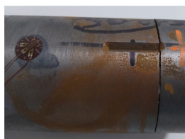
Fig. 8. Image showing the circumferential crack alignment of the only axial pit pipe that failed due to cyclic bending loading. Note that the crack passes through one end of the pit, rather than the centre.
