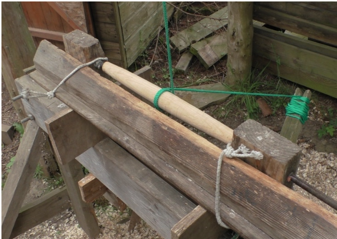
Figure 19 Photograph of pole lathe and billet of wood/stool leg
