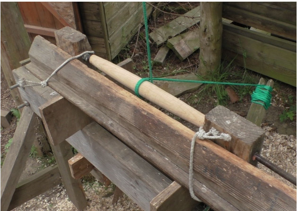
Photograph of pole lathe and billet of wood/stool leg
