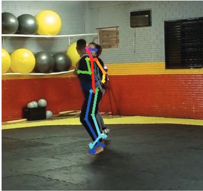
Figure 1.2 - OpenPose errors in detecting multiple people due to occlusion [5]
