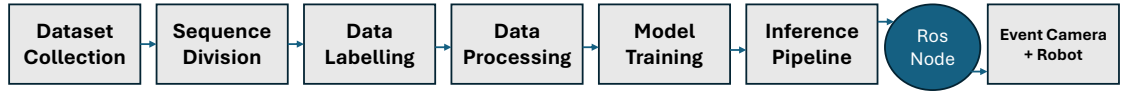
Figure 4.4: Block diagram of the proposed system. Starting with data collection to real-time gesture recognition with an event camera mounted on a robot.
