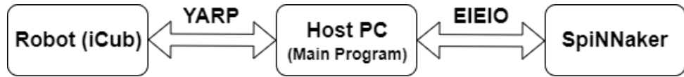
Figure 2.6: General block diagram of iCub-SpiNNaker system. The I/O from the robot is converted into YARP bottles. It is then processed by a host-based EIEIO transceiver which converts the message into spikes to transmit and receive from SpiNNaker.
