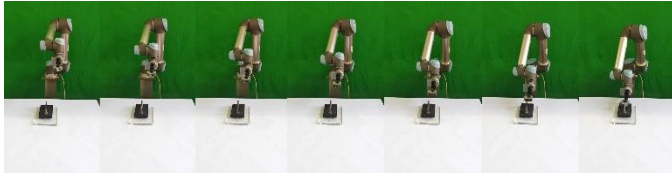
Fig. 9. The snapshots of the trained agent performed during the assembly task in the real world
