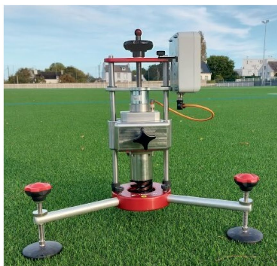
Fig. 1 The Advanced Artificial Athlete (AAA) [13]. a Left image shows a schematic of the AAA test apparatus; b Right image shows the AAA test apparatus in use in the field
