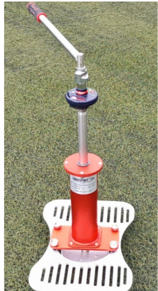
Fig. 2 The Rotational Traction Athlete (RTA) [13]; a Left image shows a schematic of the RTA; b Right image shows the RTA in use in the field
