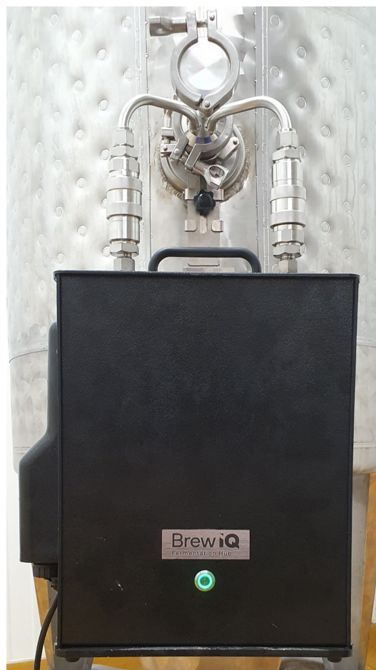
Figure 4. BrewIQ fermentation sensor array used to collect inline temperature, Plato, and pH measurements.
