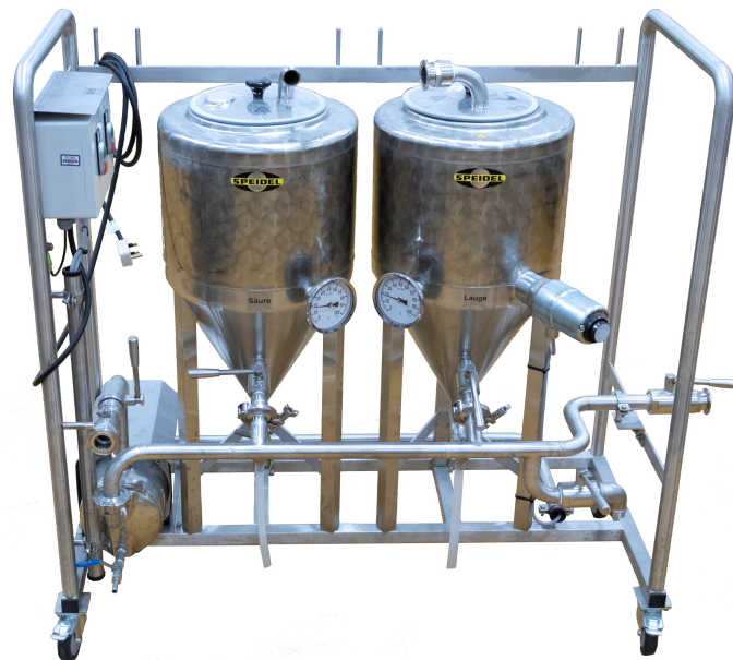
Figure 3. The Speidel clean-in-place (CIP) apparatus used to clean and sanitise the 240 L fermenter (Figure 2).
