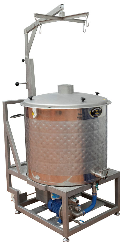
Figure 1. The 200 L Speidel's Braumeister brewhouse used to produce the IPA-style wort.
