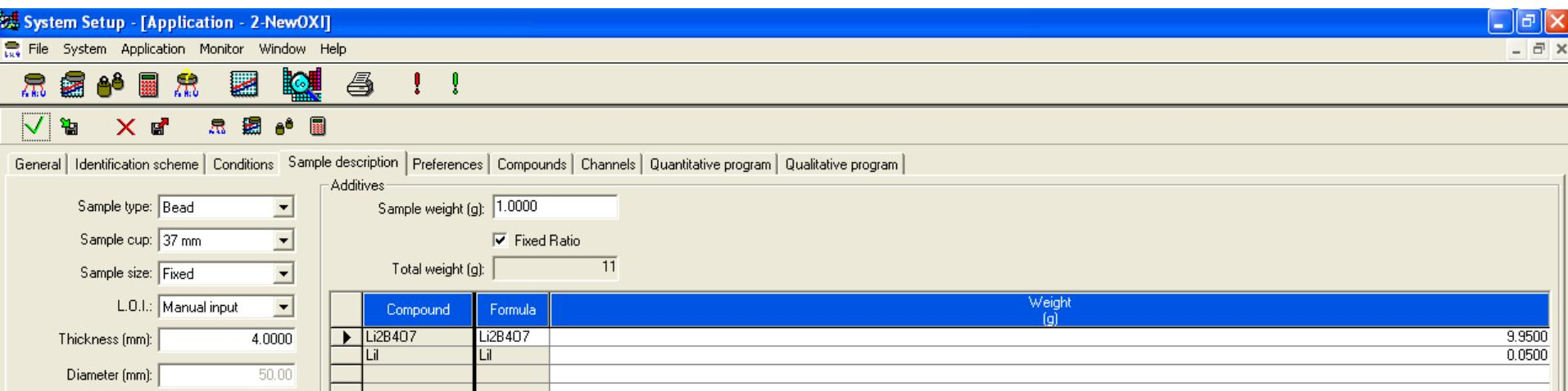
The screenshot shows the 'System Setup - Application - 2-NewOXI' window. The 'Additives' tab is selected. The 'General' tab is also visible. The 'Sample type' is set to 'Bead'. The 'Sample weight (g)' is 1.0000. The 'Total weight (g)' is 11. The 'Fixed Ratio' checkbox is checked. The 'Compound' table lists Li2B4O7 and LiI with their respective formulas and weights: Li2B4O7 (9.9500 g) and LiI (0.0500 g).
