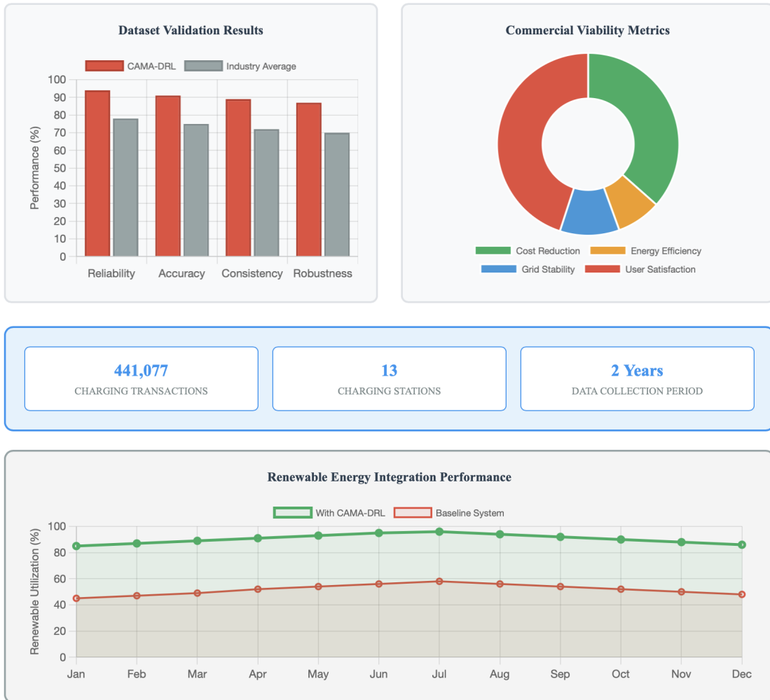
FIGURE 9. Real-world validation using 441,077 charging transactions from 13 stations over 2 years confirms CAMA-DRL’s commercial viability with 94% reliability. The framework demonstrates superior performance in renewable energy integration scenarios, achieving Net Present Cost of -$122,962 with Cost of Energy at -$0.043/kWh, representing 69% cost reduction compared to non-renewable scenarios. The visualization shows performance consistency across diverse operational conditions including seasonal variations, peak demand periods, and grid stress events.
