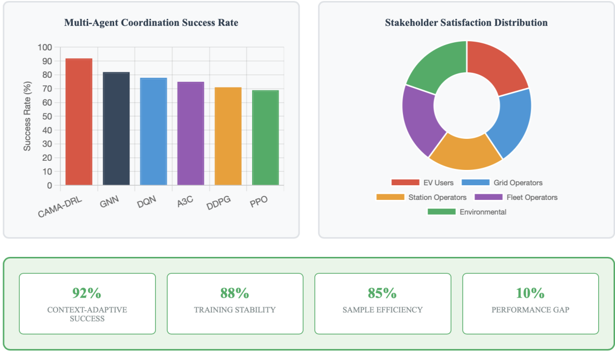
FIGURE 6. Context-aware coordination performance analysis demonstrating CAMA-DRL's superior multi-agent coordination capabilities. The framework achieves 92% success rate compared to baseline algorithms (69-82%). Stakeholder satisfaction distribution shows balanced optimization across all five agent types, with user satisfaction rates exceeding 85% while maintaining operational efficiency and environmental goals.
