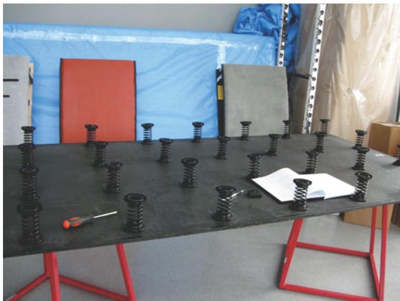
Figure 1. Underside of a spring floor panel using steel coil springs.
