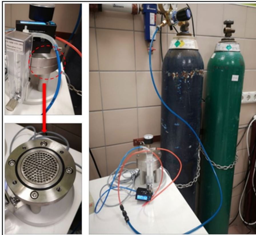
FIGURE 3 | Gas permeability test setup.
