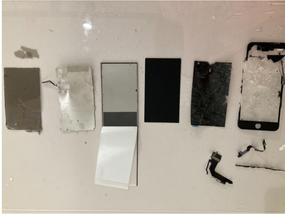
Figure 28. Figure of the work in progress of delayering and discovering the touchscreen layers.
