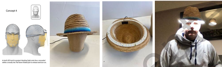
Figure 8. The 'halo hat' with a ring of LED around the brim. The on-off control is a simple switch.
