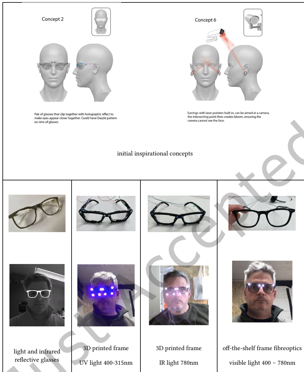
Figure 6. The concepts of morphing glasses and a camera-attack mechanism that inspired the design of glasses projecting out.
