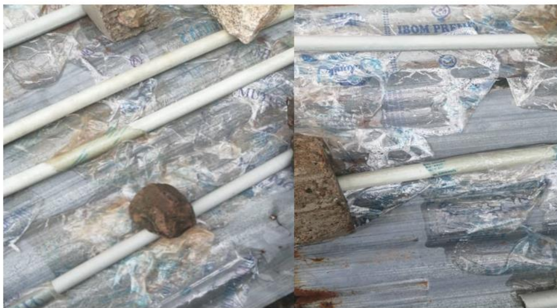
Figure 4. 20: A selection of the PE water sachets spread on the aluminium zinc, directly exposed to the sunlight, and supported with plastic pipes and stones to avoid being blown away by the wind
