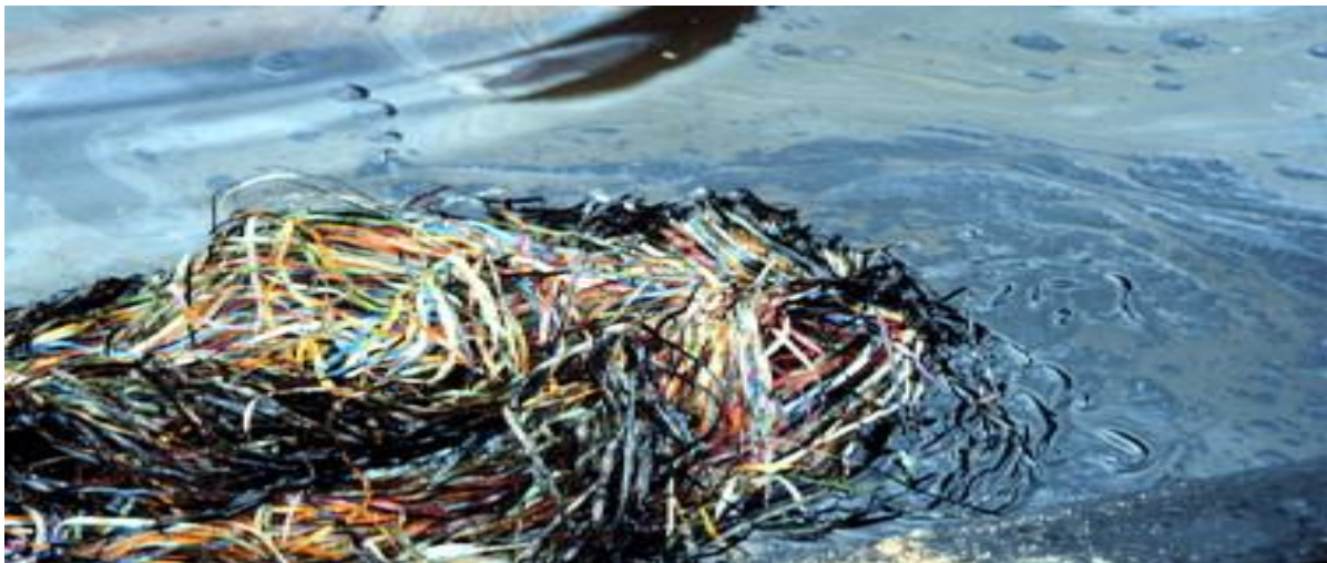
Figure 2. 6: Pom poms fibres attract and hold heavy oils used in the Exxon Valdez oil spill
