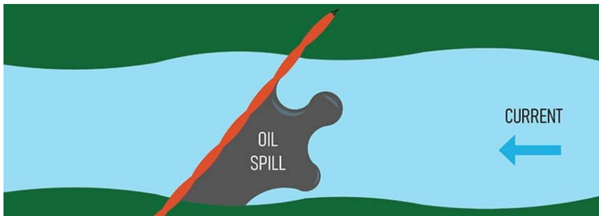
Figure 2. 1: How oil spill containment boom contains spilt oil on water
