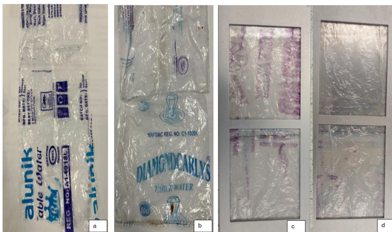
Figure 4. 26: (a) Pristine PE (b) Naturally weathered PE for 50 days (1200 hrs) (c) UV-weathered PE for 75 hours (d) UV-weathered PE for 150 hours
