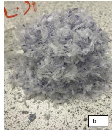
Figure 4. 28: (a) Shredded PE consisting of large flakes body with elongated strands (b) Shredded-roughened PE
