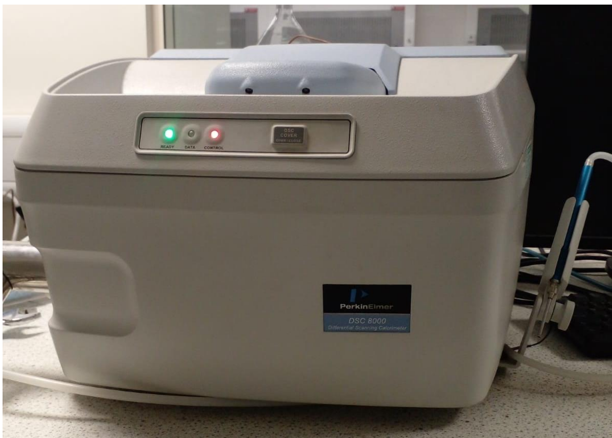
Figure 3. 12: Differential Scanning Calorimetry (DSC) for Thermal analysis
