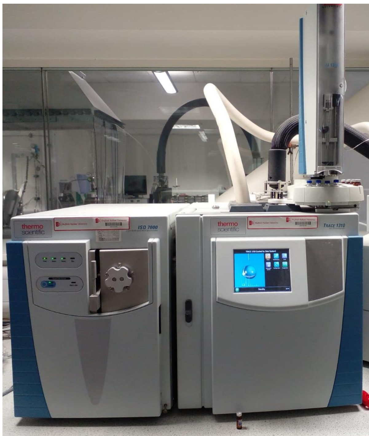
Figure 3. 6:GCMS (ThermoScientific Trace 1310 Gas chromatograph: ISQ 7000 Single Quadrupole Mass Spectrometer)
