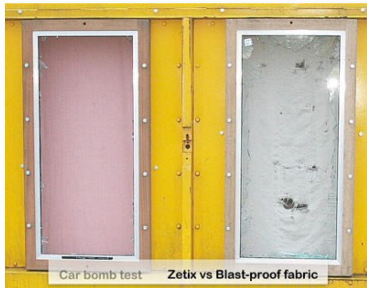
Figure 18: Comparison of Zetix blast curtain (left) with conventional blast-proof material (right) after the blast test conducted by the UK Ministry of Defence (TextileWorld, 2010)
