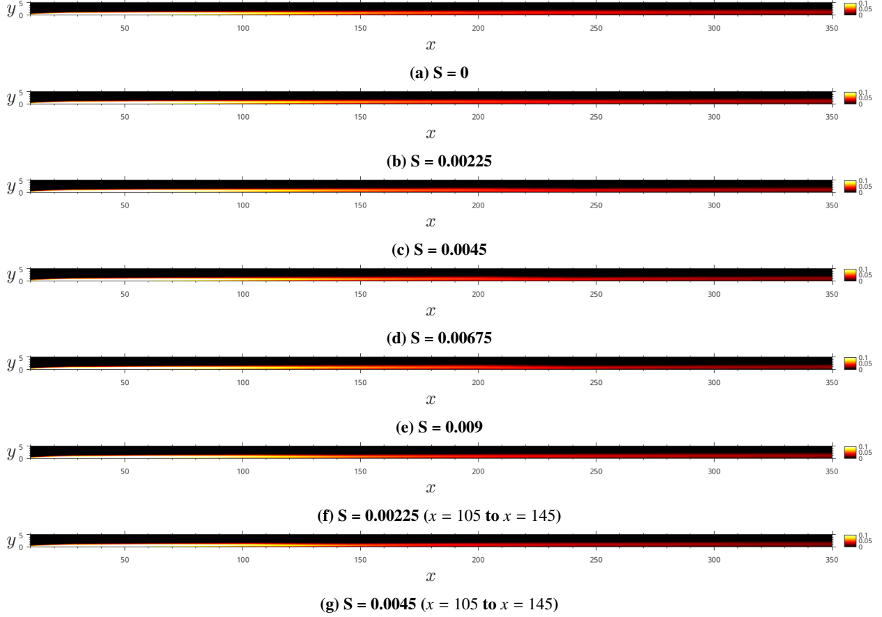
Fig. 20 Midspan Coolant mass fraction contours for various suction ratios (Wall-normal: XY Plane)
