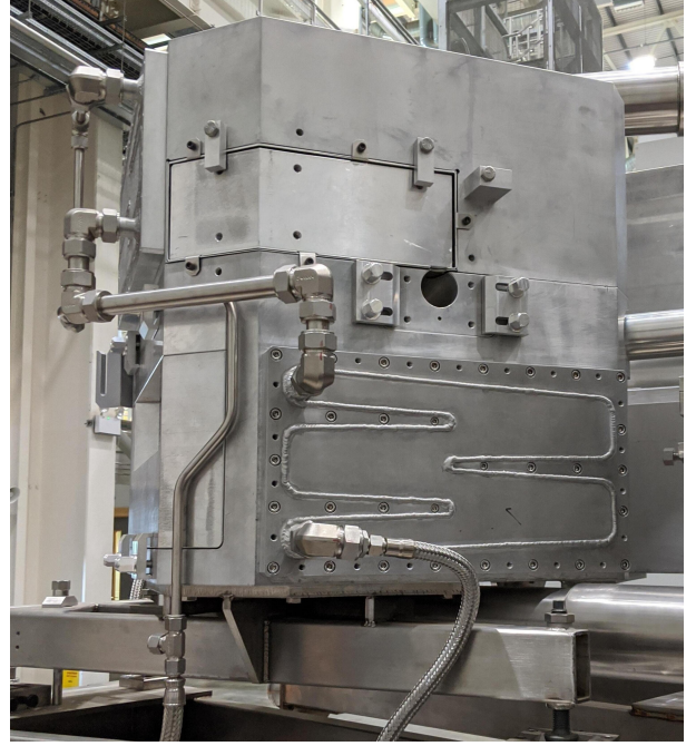
(b) The aperture that guides fast neutrons to the ChipIr irradiation chamber. This photo is taken at approximately 120^\circ (anticlockwise) offset to the direction of the photo in Figure 6.1a
