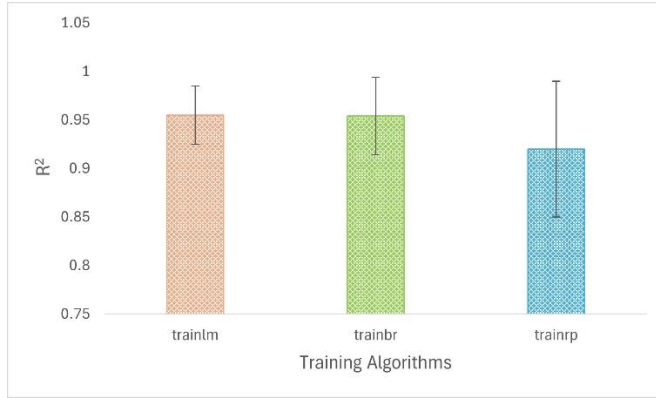
Figure 5: Average test R^2 achieved by each training algorithm ( trainlm : Levenberg–Marquardt, trainbr : Bayesian regularisation, trainrp : resilient backpropagation).
