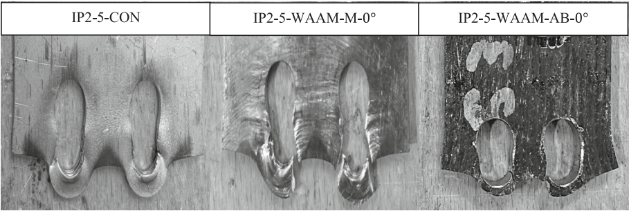
Fig. 18. Failure modes for IP2-5 configuration of CON and AM plates.
