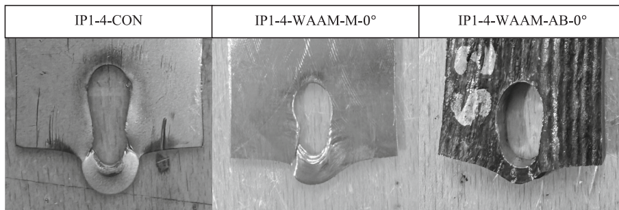
Fig. 12. Failure modes for IP1-4 configuration of CON and AM plates.
