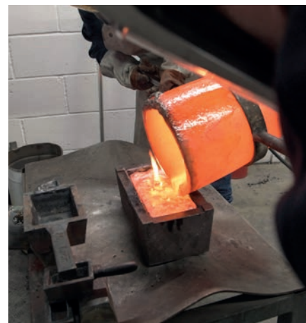
◀ The molten silver is poured into a mould. Sheffield, November 2021
