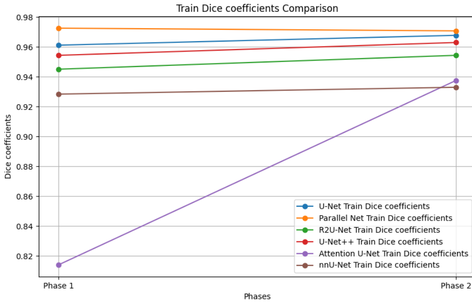
FIGURE 8. Best train dice coefficients comparison graph for UNet, Parallel Net (MPNET), R2U-Net, U-Net++, Attention U-Net, and nnU-Net over two validation phases.
