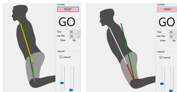
Fig. 1 Custom-made visual feedback system, and on-screen mannequin with reference line. The moving reference line turns orange (a) as a warning if within a range of 5^\circ and then red if greater than 5^\circ from the set coordinates
