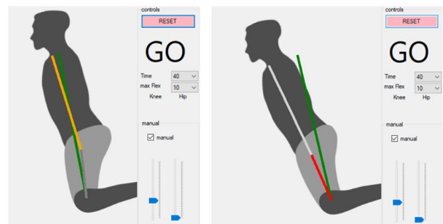
Fig. 1 Custom-made visual feedback system, and on-screen mannequin with reference line. The moving reference line turns orange (a) as a warning if within a range of 5^\circ and then red if greater than 5^\circ from the set coordinates
