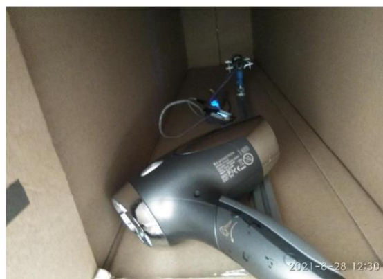
Figure 2.8: A domestic hair dryer used for preferred change temperature steps.
