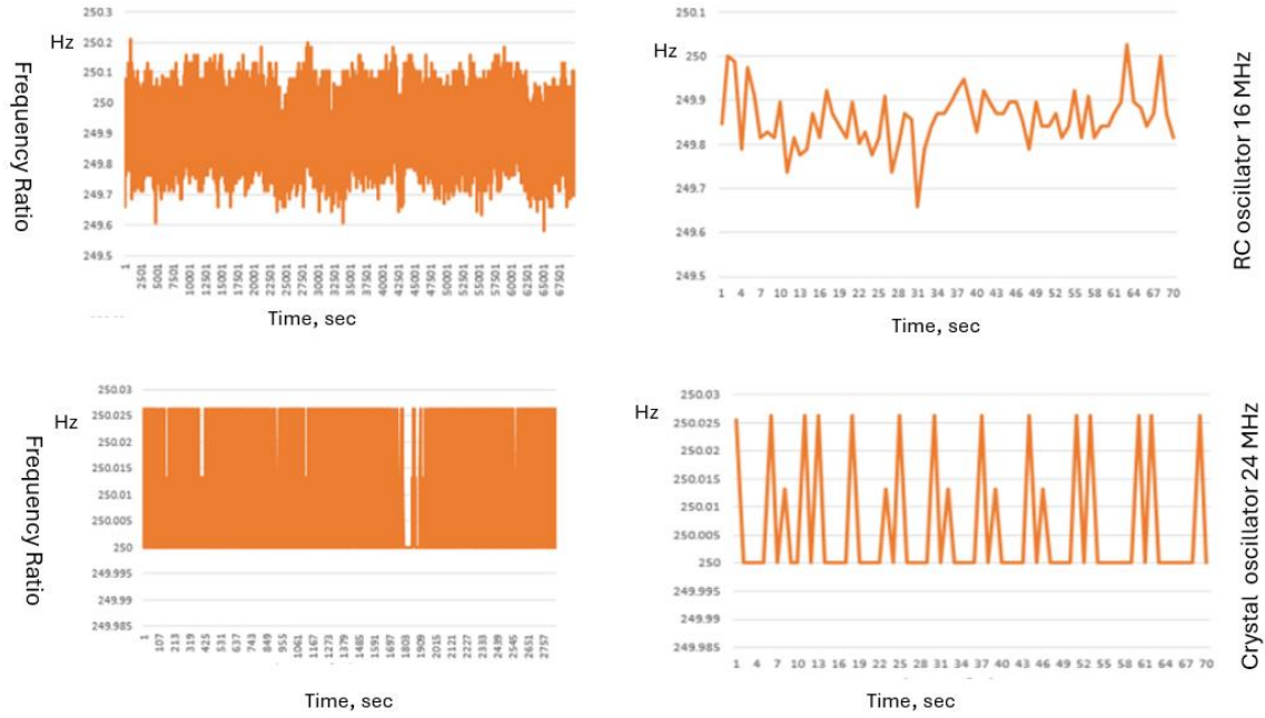
Figure 2.16: Measured ratios Fr/Fx for 40 periods of Fx (100 ms delay between measurements)
