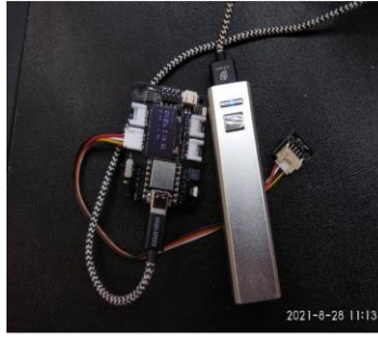
Figure 3.5: Conventional temperature sensors AHT20, BMP280 and SD card adapter.
