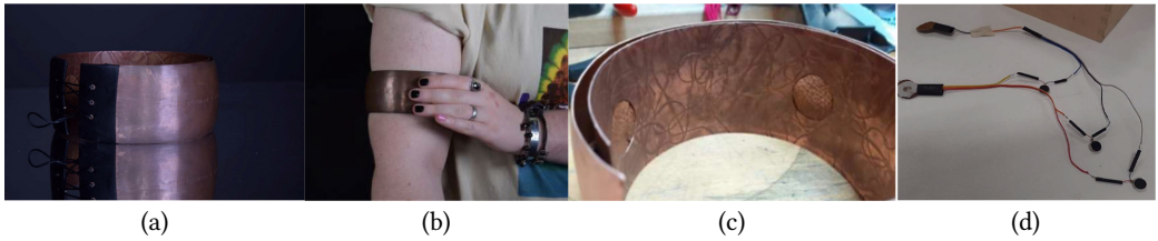
Fig. 8. Amulet for Anxiety is a digital bracelet that vibrates when touched. A personal affirmation text is engraved on the outside (a). The piece is made of copper, leather and electronics (vibration motors, touch sensors, battery) (a, b). The circuitry is encased within two sheets of copper; holes in the inside of the metal sheet secure the vibrator motors, covered in leather (c). The vibration of the amulet is activated by pressing two touchpads (b, d) and could be fastened more tightly by pulling the strings (a).
