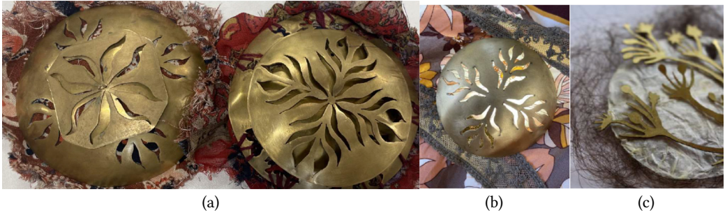
Fig. 7. Connected Brooches are a pair of connected digital brooches for two wearers. When the top layer of one brooch is spun, the other brooch lights up; initially low, the light increases in intensity as the spinning intensifies. From left to right: (a) Final form of the brooches in brass and fabric. The electronics assemblies a potentiometer for each brooch, a microcontroller with WiFi connection, LED light and a LiPo battery. (b, c) Explorations of form and light: metal and fabric; metal, papier-mâché and human hair.
