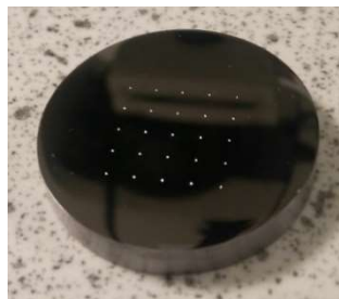
Figure 4.3 Image of polished tantalum sample after Vickers hardness test under the load of 2 kgf on 25 indents (5 x 5 matrix) visible on the sample surface.
