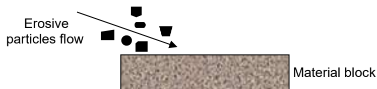
Figure 2.1 Erosive particles of various shapes/sizes striking the material block at a specific angle/velocity.
