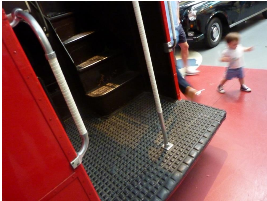
Figure 5.7: Textures of the rear platform. Required for the safe negotiation of entry and exit, the white grip sections particularly evocative and expressive of the specific motion performed by millions of Londoners daily.
