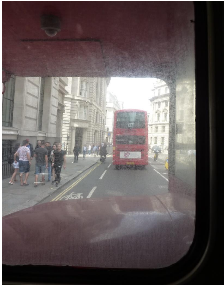
Figure 5.11: Unwashed windows of the 15(H) service. Inaccessible by contemporary automated bus-washers.
