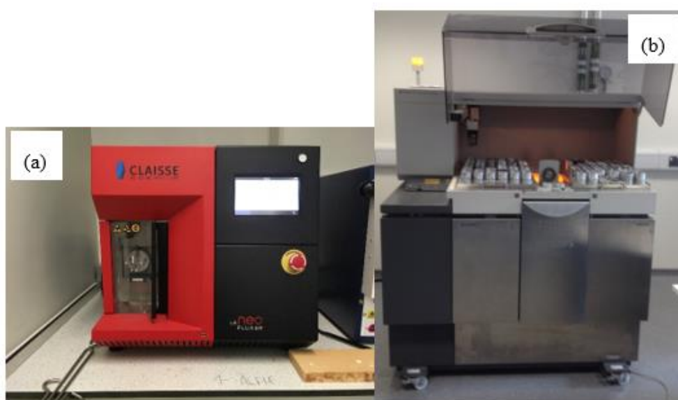
Figure 3-4: (a) XRF fused bead maker and (b) Phillips MagiX Pro X-Ray fluorescence spectrometer analyser at SHU
