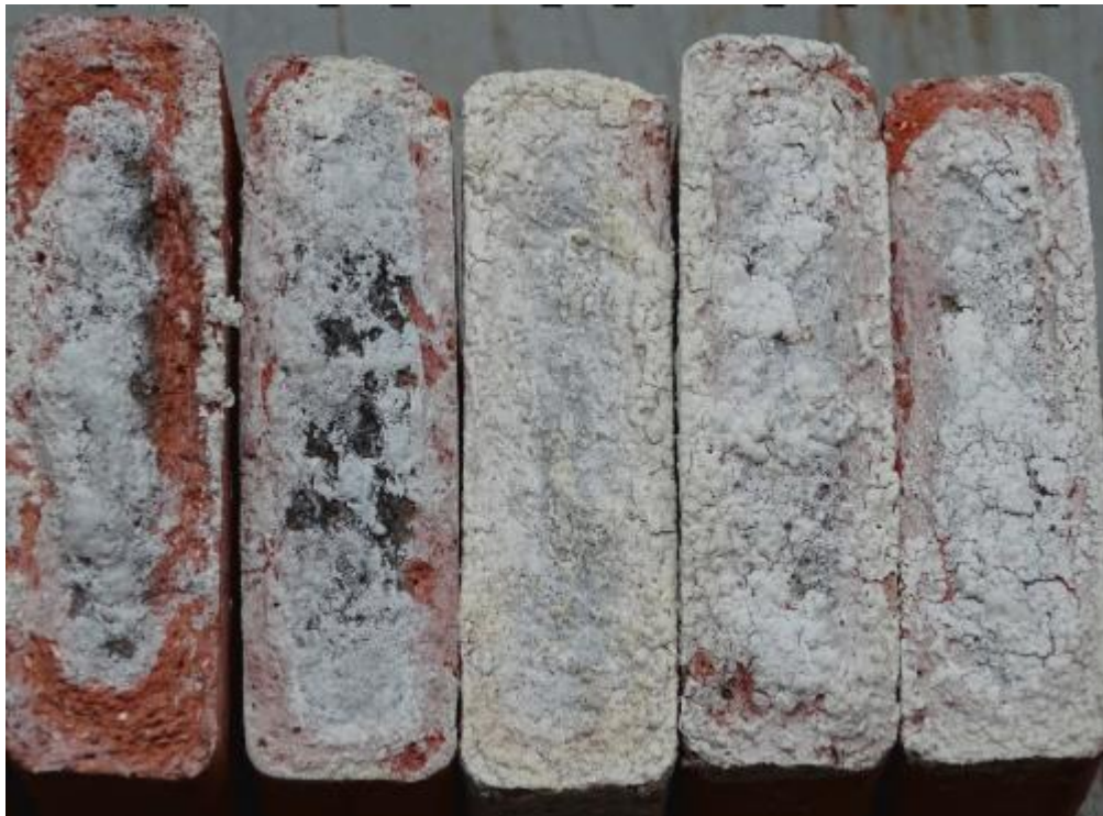
Figure 2-16: Effloresced ceramic containing sulphidic mine waste fired to 965°C 73 .
