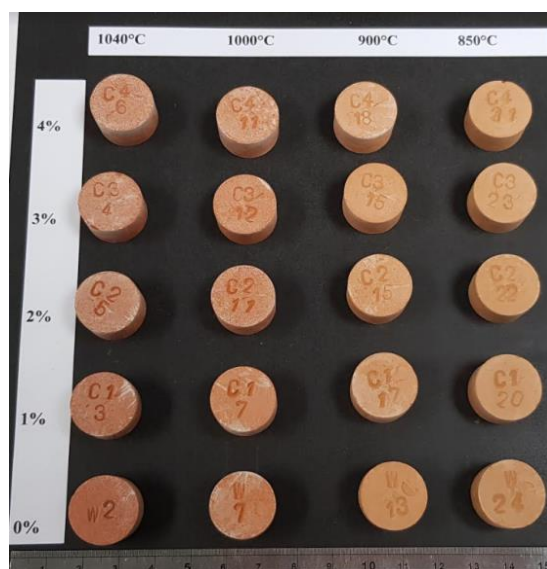
Figure 5-51: Comparison of fired images of baseline to 1-4wt% \text{CaCO}_3 additives fired to 850°C, 900°C, 1000°C and 1040°C
