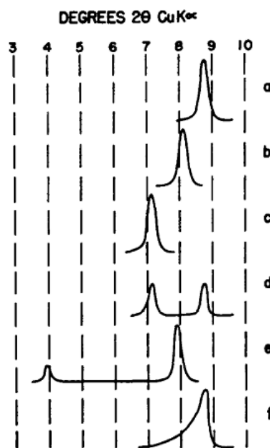
Figure 2-10: Powder diffraction of low angle 1M muscovite and montmorillonite clay mineral (taken from Yoder and Eugster 104 )
