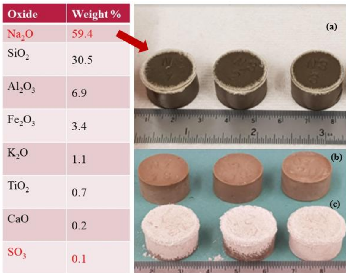
Figure 8-13: Whitish substance forms on Weald clay containing Na 2 CO 3 additive (a) Wet clay sample with developed efflorescence after adding 3wt% Na 2 CO 3 (b) Dry clay shaped sample containing 1wt% Na 2 CO 3 and (c) bench drying of Na 2 CO 3 containing the sample and its bulk chemical composition with XRF.
