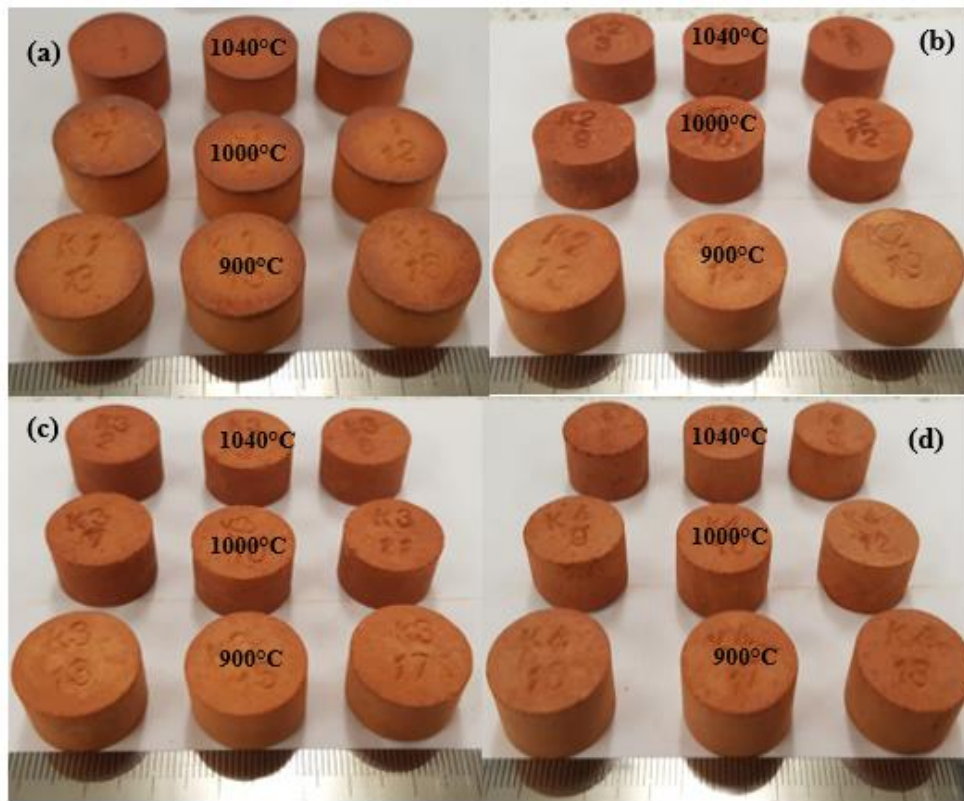
Figure 8-2: Surface defects of ceramic samples containing K_2CO_3 fired to 900°C-1040°C (a) 1wt% K_2CO_3 darker -patches at the rim(b) 2wt% K_2CO_3 lighter shade patches (c) 3wt% K_2CO_3 lighter shade patches and (d) 4wt% K_2CO_3 lighter shade patches.
