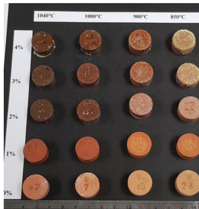
Figure 5-56: Comparison of fired images of baseline to 1-4wt% Na_2CO_3 additives fired to 850°C, 900°C, 1000°C and 1040°C
