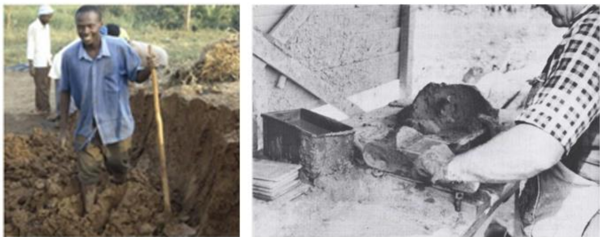
Figure 2-2: Clay preparation- “the naked feet” approach 33 and shaping clay brick in a wooden mould 6
