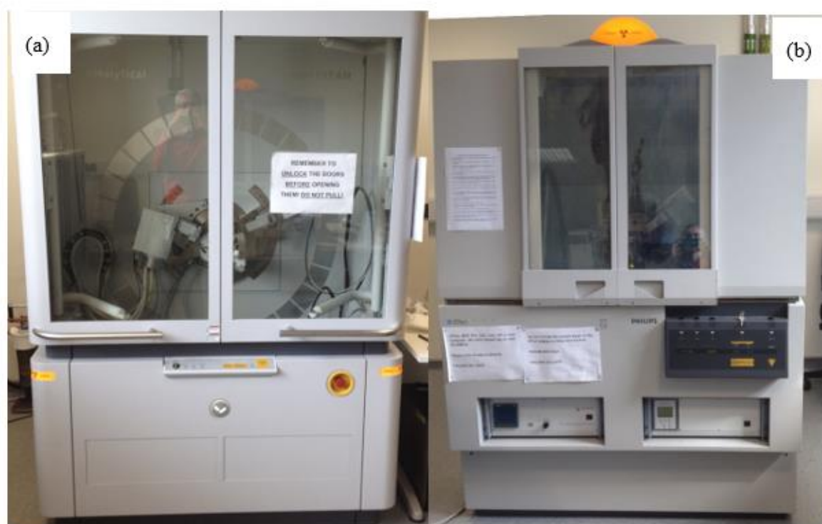
Figure 3-6: XRD equipment at SHU (a) Empyrean using a Co anode X-ray source and (b) X'Pert using a Cu anode X-ray source.
