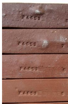
Figure 2-18: Bloated ceramic distorting ceramic shape 210
