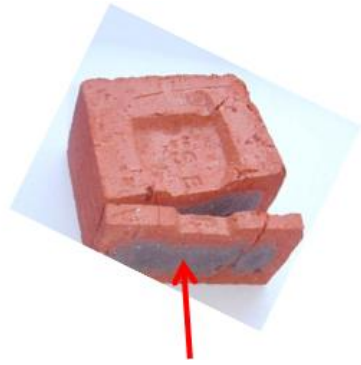
Figure 2-17: source Gredmaier et al., 151 Black core a significant problem in heavy clay brick manufacture.
