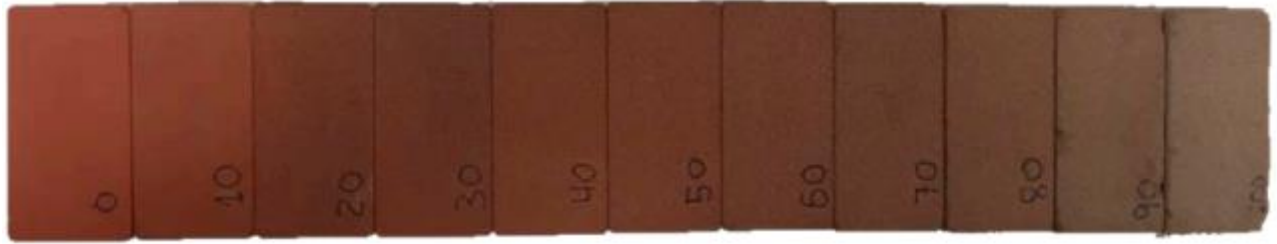
Figure 2- 1: The effect of mining waste on brick colour as levels increased from 10-100% and the mixture fired to 950°C for 1hr at a heating rate of 4°/min 251 .
