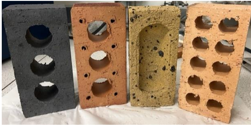
Figure 2-12: Created holes and frogs in some Wienerberger-fired brick products for material reduction.
