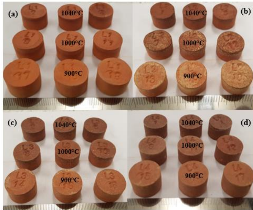
Figure 8-1: Surface defects of ceramic samples containing \text{Li}_2\text{CO}_3 fired to 900°C-1040°C (a) 1wt% \text{Li}_2\text{CO}_3 (b) 2wt% \text{Li}_2\text{CO}_3 dark rim and creamy-yellowish patches, (c) 3wt% \text{Li}_2\text{CO}_3 and (d) 4wt% \text{Li}_2\text{CO}_3 darker rim and creamy-yellowish patches/melts
