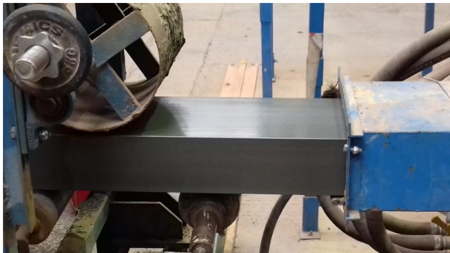
Figure 2-5: Extrusion of clay brick at Wienerberger's factory site (Ewhurst, UK)
