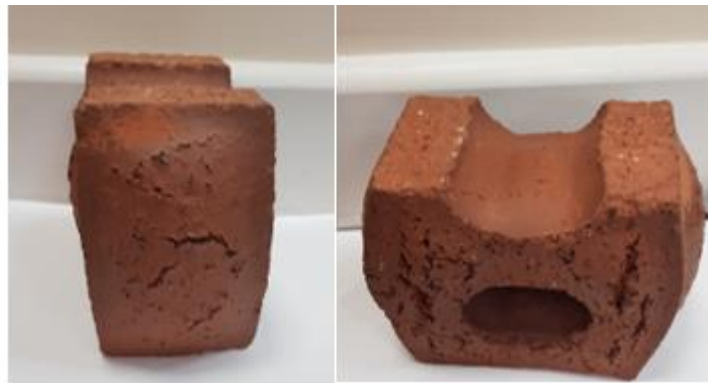
Figure 2-19: Overfired heavy clay product
