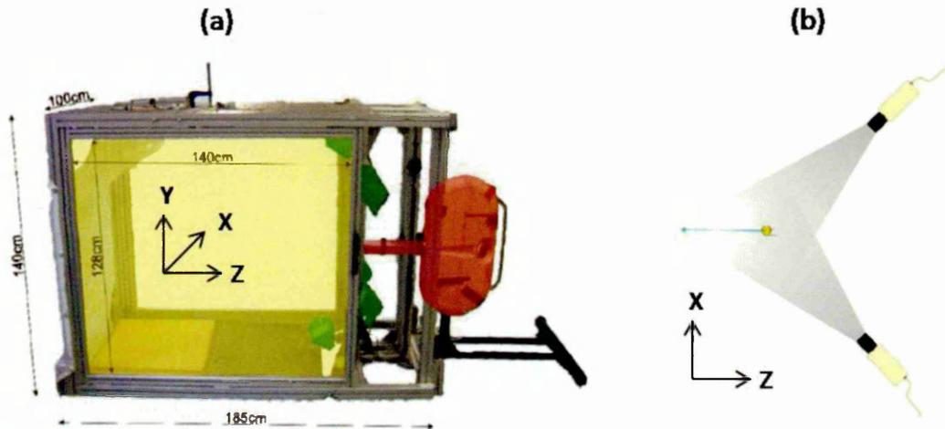
**Figure 5.5** a) Impact rig used for simulating impacts on a freely suspended tennis racket (Modified from Choppin, 2008) b) Optimum camera positions for measuring the trajectory of a tennis ball in 3D (Modified from Choppin, 2008).
