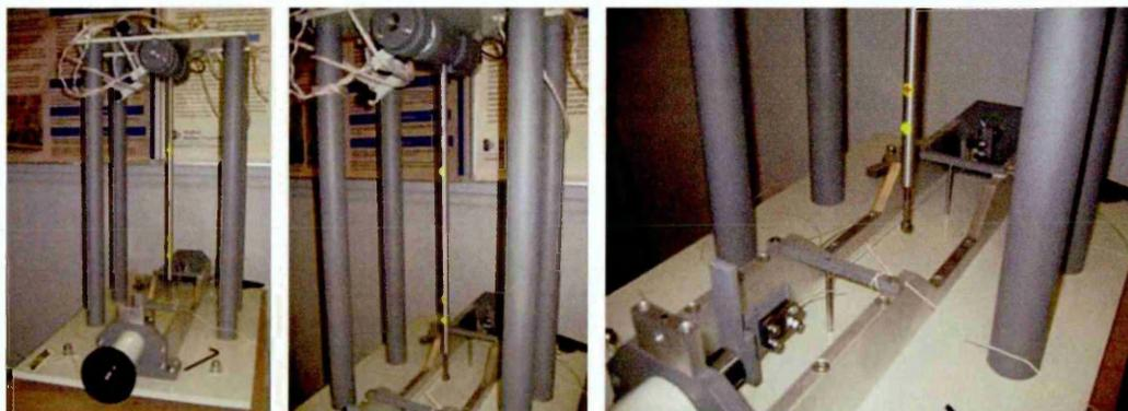
**Figure 1.23** Modified impact rig (Hammer head replaced with bolt)
