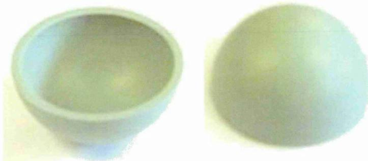
**Figure 3.1** Hemispherical rubber cores provided for material testing.
