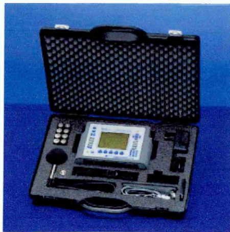
Figure 7.14 : The NC10 Analyser, microphone and calibrator
