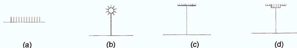
Figure 3.14 : Barriers with reactive surfaces (a) series of parallel ribs on the ground, (b) waterwheel, (c) constant depth reactive T-capped barrier, and (d) variable depth reactive T-capped barrier.
