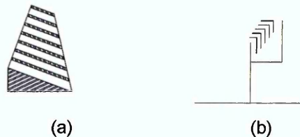
Figure 3.10 : Interference based noise barriers (source to the left)
