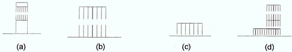
Figure 3.11 : Phase reversal barriers (a) slow – waveguide, (b) basic dipolar type, (c) halfguide dipolar type, and (d) quadrupolar type
