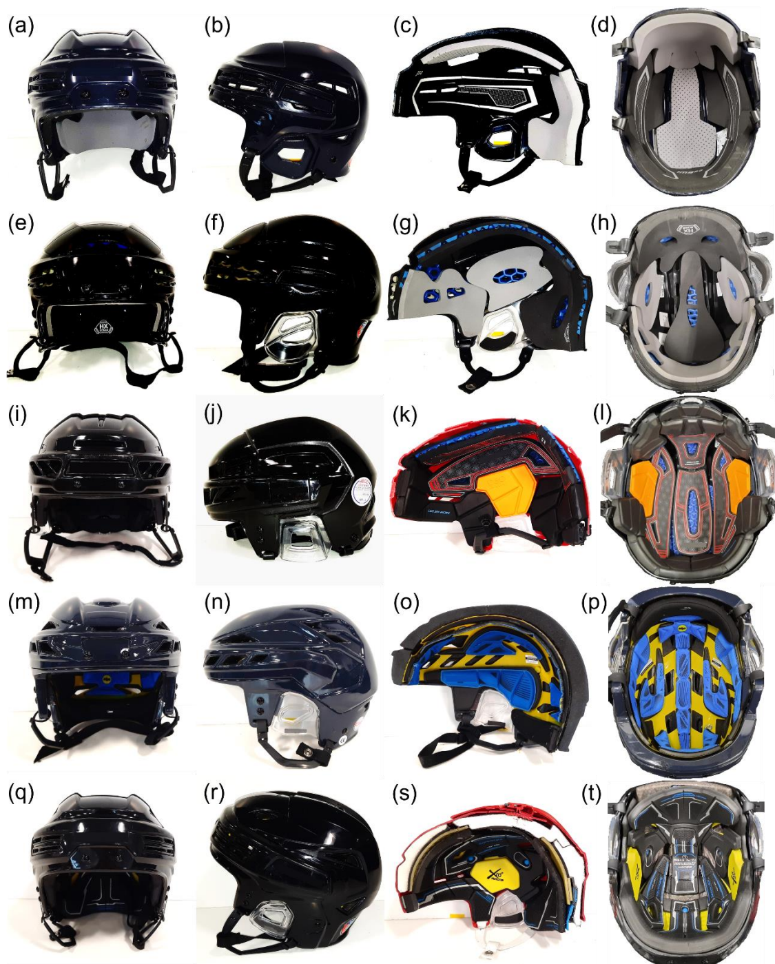
Fig. S1 Helmet shells and liner systems for helmet (a - d) 1, (e - h) 2, (i - l) 3, (m - p) 4, and (q - t) 5
