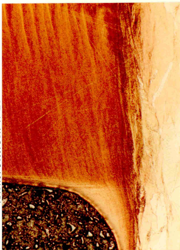
FIGURE 74 PHOTOMICROGRAPHS OF THE CHIP ROOT AREA WHEN CUTTING COPPER WITH BLUNT TOOLS (0,56 MM RADIUS) (NOMINAL SET DEPTH - 0,25 MM)
