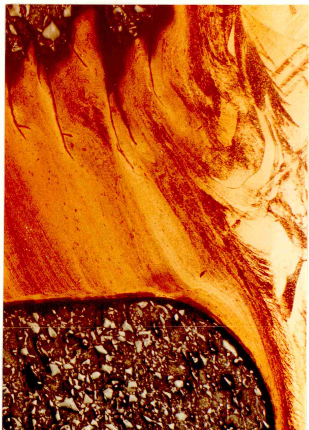
FIGURE 74 PHOTOMICROGRAPHS OF THE CHIP ROOT AREA WHEN CUTTING COPPER WITH BLUNT TOOLS (0,56 MM RADIUS) (NOMINAL SET DEPTH - 0,25 MM)
