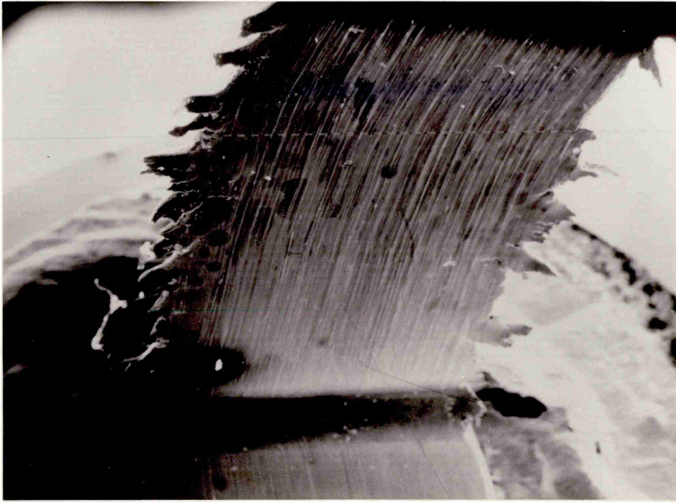
FIG.75 ELECTRON-MICROSCOPE PICTURE OF THE CHIP ROOT AREA
