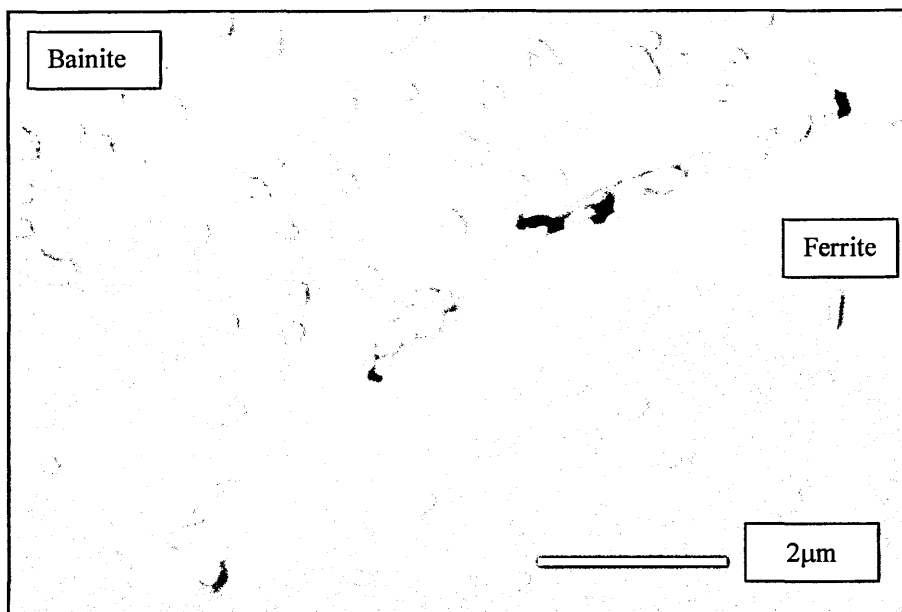
Plate 4.41: SEM image depicting cavitation on a ferrite / bainite grain boundary and growth of associated grain boundary carbides. PFZ evident in the ferrite grain adjacent to the grain boundary.
