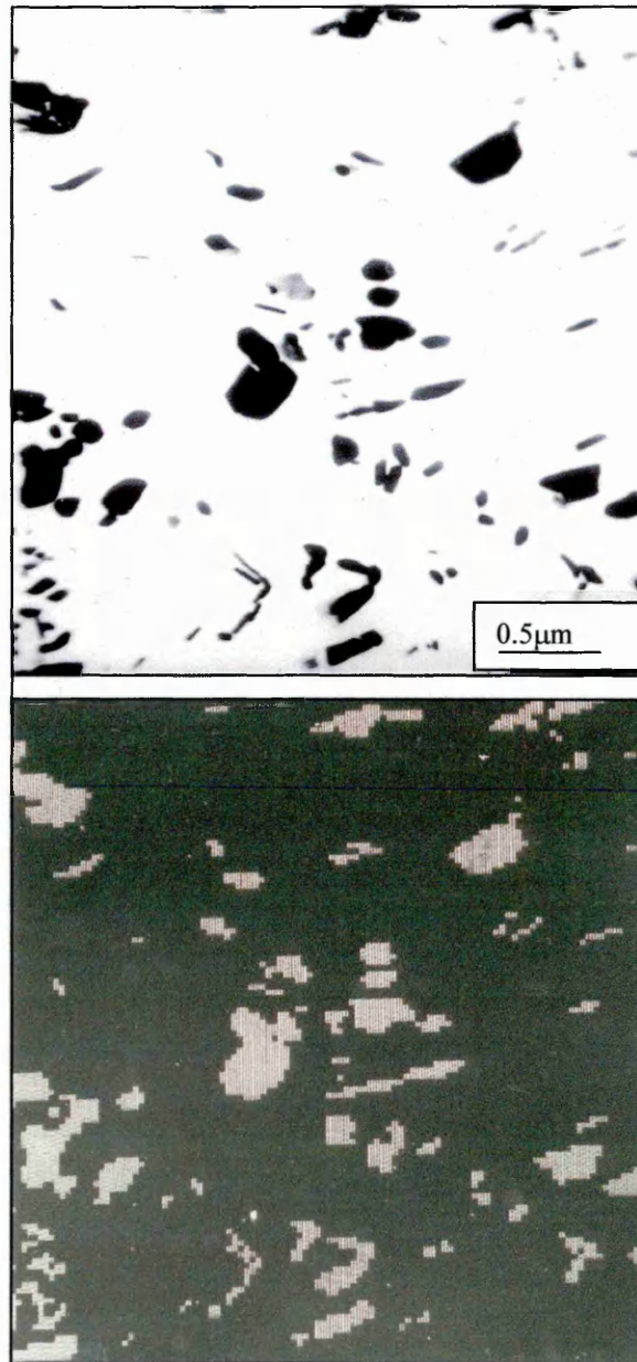
Figure 3.9: STEM images of a) carbide precipitates and b) the corresponding digitised image.
