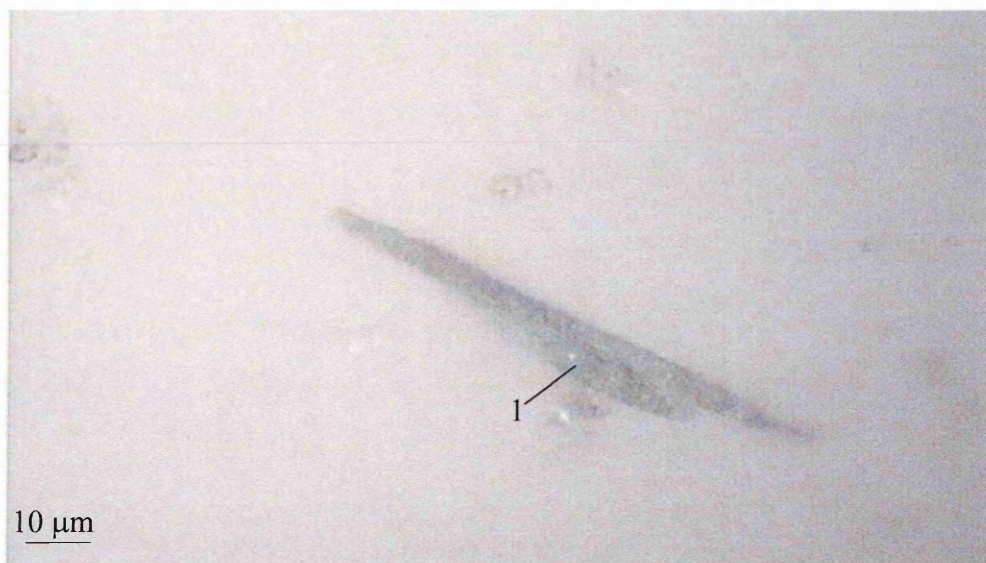
Figure 6.11: Micrograph of a wet crocidolite fibre on cellulose filter.
