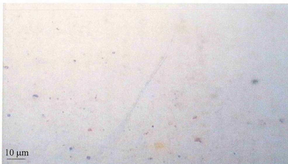
Figure 5.13: Micrograph of particles and fibres from 'real industrial sample' on cellulose filter.
