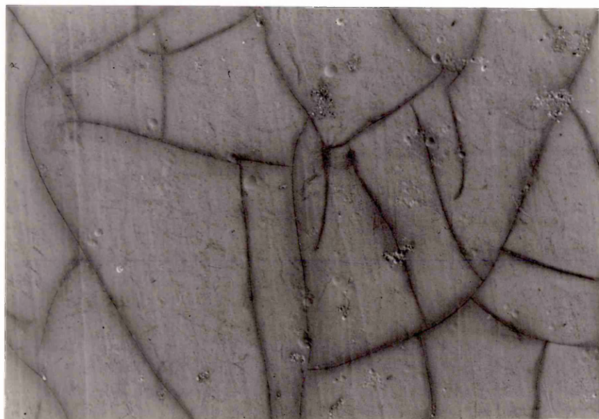
Fig. 4-2: Surface Morphology of Deposit Produced in NiFe Solution 4 at 30 \text{ mA cm}^{-2} .
