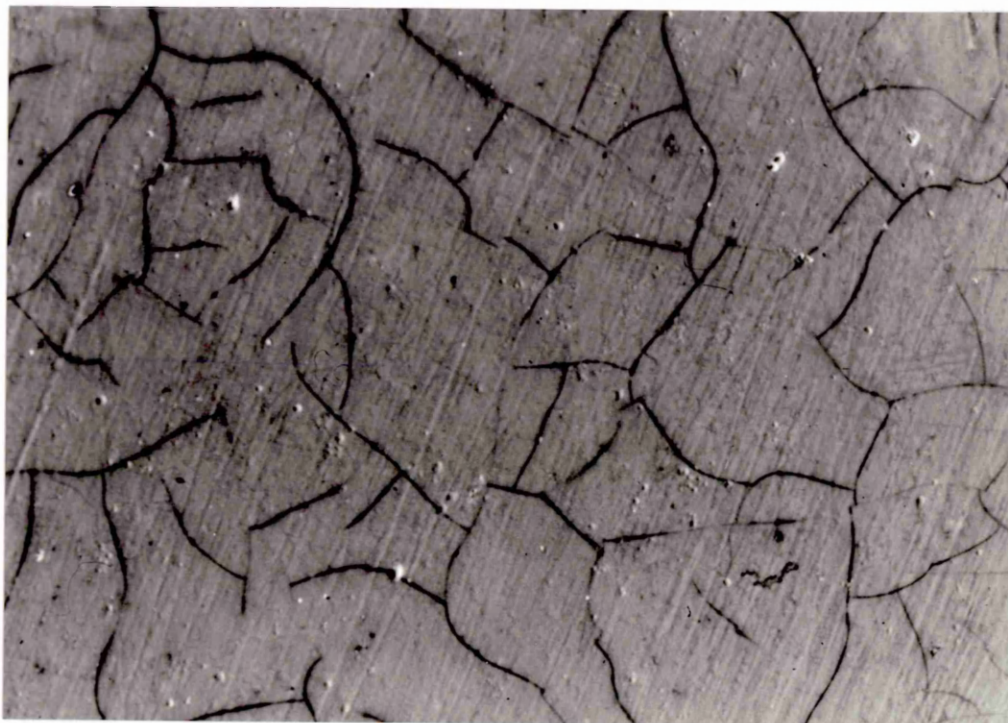
Fig. 4-1: Surface Morphology of Deposit Produced in NiFe Solution 4 at 10 \text{ mA cm}^{-2} .
