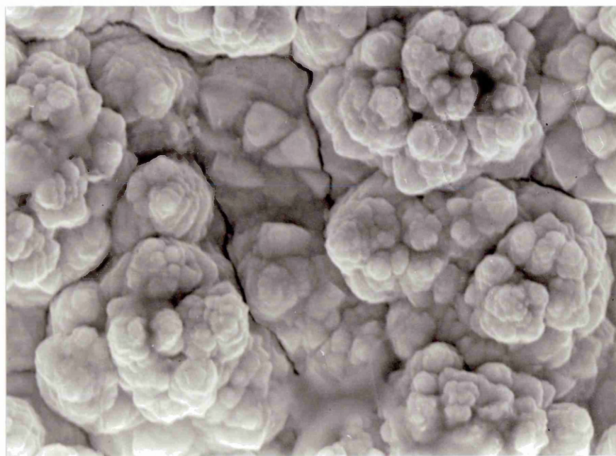
Fig. 4-4: Surface Morphology of Deposit Produced in NiZn Solution 8 at 10 \text{ mA cm}^{-2} .
