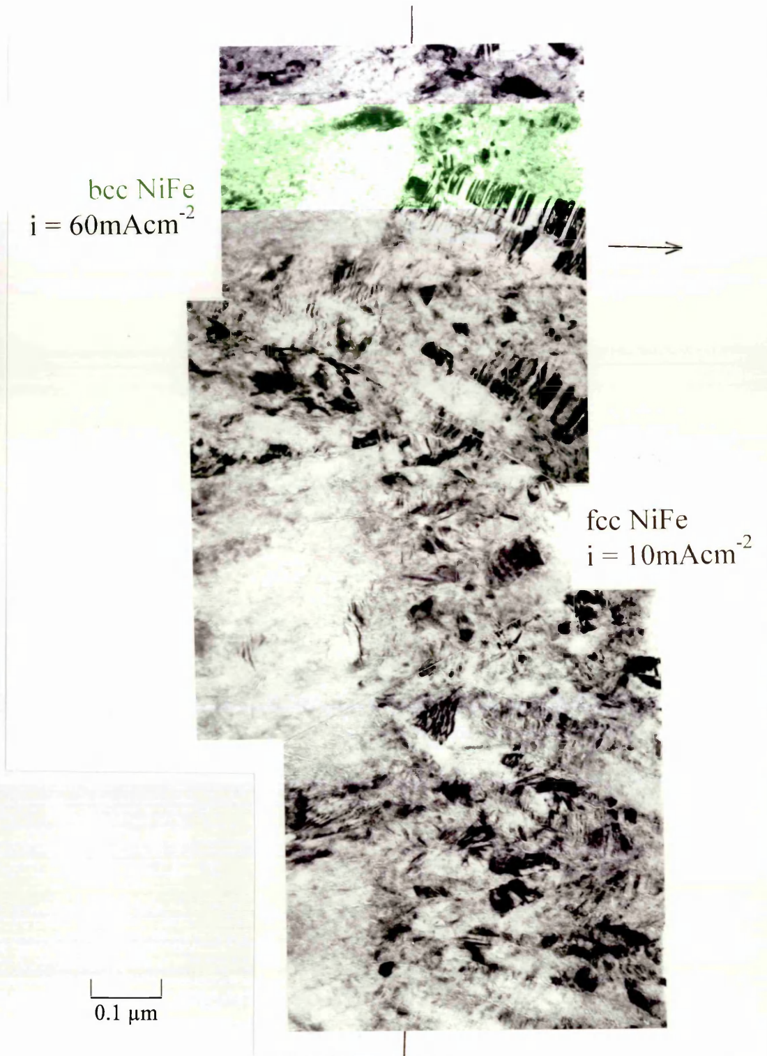
Fig. 4-61: Montage of Bright Fields Along Interface of Double Layered 2\mu\text{m} Thick fcc NiFe Deposit Nucleated on 2\mu\text{m} Thick bcc NiFe Deposit.
