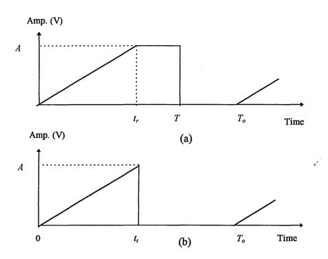
Fig. 3.8 PSM pulses waveforms: (a) trapezoidal and (b) triangular.
