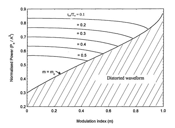
Fig. 3.10 Normalised average power of trapezoidal PSM signal ( $T/T_0 = 0.9$ )
