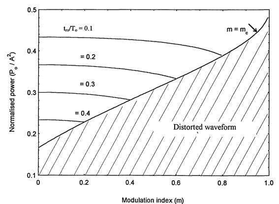
Fig. 3.11 Normalised average power of trapezoidal PSM signal ( $T/T_0 = 0.5$ ).
