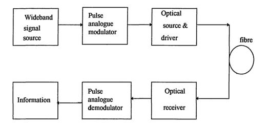
Fig. 2.5 Pulse analogue modulation system.
