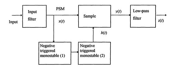
Fig. 3.6 Block diagram of the proposed PSM demodulator.
