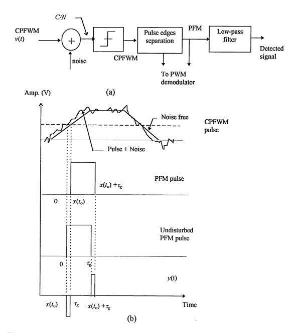
Fig. 7. 27 PFM demodulator with noise: (a) block diagram and (b) waveforms.
