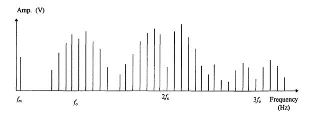
Fig. 2.19 Frequency spectrum of a PFM signal.
