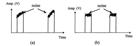
Fig. 3.18 (a) Pulses at the sampler output when modulation is absent and (b) pulses considered by Jelonek [25].
