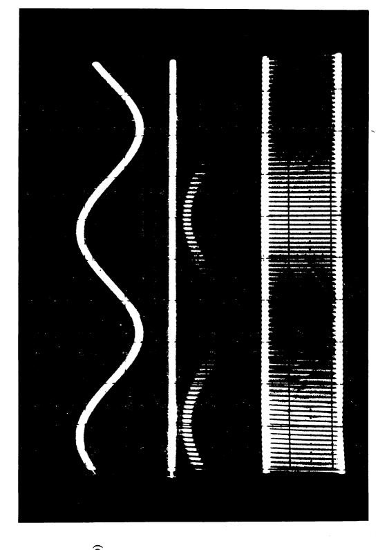
Fig. 3.23 Waveforms at the PSM receiver: (a) PSM (b) PAM and (c) detected signal (Scale 200 msec/div)
