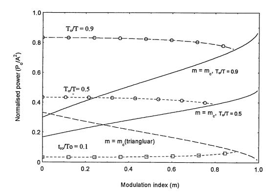
Fig. 3.13 Normalised transmitted power for both types of PSM pulses ( $t_{ro}/T_o = 0.1$ ,  $\Box$  triangular PSM,  $\circ$  Trapezoidal PSM).
