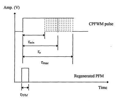
Fig. 5.9 Waveforms at the PFM pulse separation.
