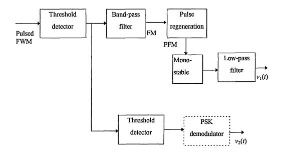
Fig. 4.17 Pulsed FWM receiver.
