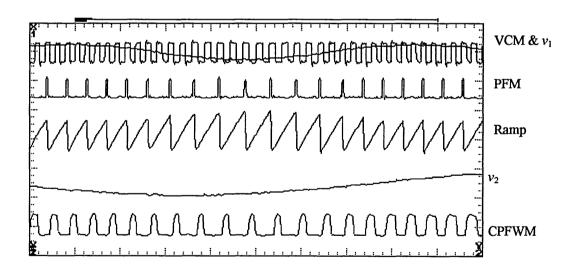
Fig. 5. 28 Recorded waveforms at the CPFWM, when both modulating signals are exist ( $\beta = 1, M = 5\%, f_1 = 130$  kHz,  $f_2 = 60$  kHz).
