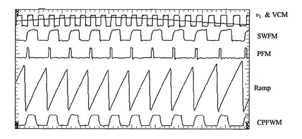
Fig. 5. 26 Recorded waveforms at the CPFWM, when  $\beta = 1$  and  $f_1 = 130$  kHz, and width modulation is absent (M = 0).
