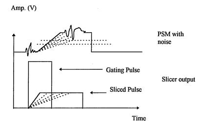
Fig. 3.17 Reduction of noise by slicing and gating.
