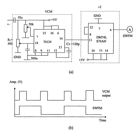
Fig. 5.15 SWFM generator: (a) circuit diagram and (b) waveforms.
