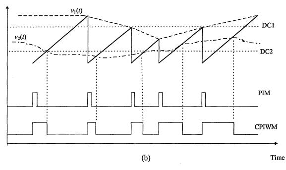
Fig 4.10 CPIWM transmitter: (a) block diagram and (b) waveforms.
