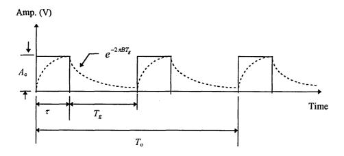
Fig. III.1 Time diagram of TDM-PPM waveform.
