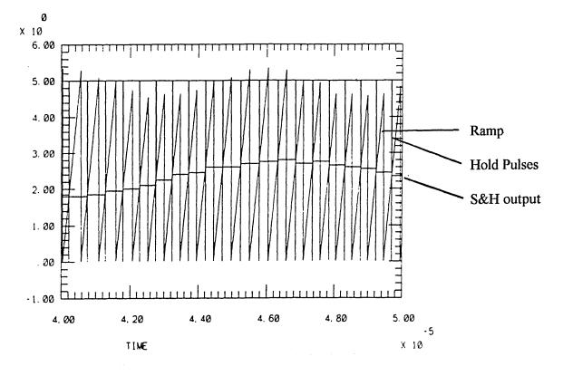
Fig. 5.13 Waveforms of CPFWM receiver.
