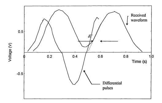
Fig. 7.2 Received CPFWM waveform of dual pulses and its slope.
