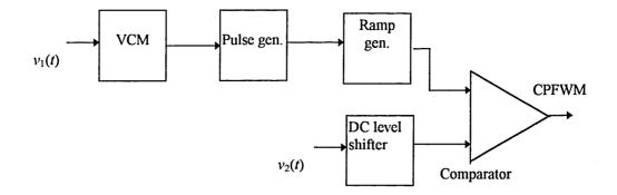
Fig. 7.1 Simplified block diagram of CPFWM transmitter.
