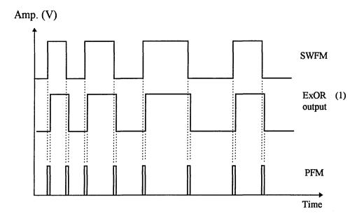
Fig. 2.23 Double edge SWFM detection waveforms.
