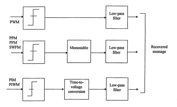
Fig. 2.25 The basic PTM demodulation techniques.
