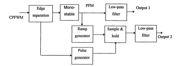
Fig. 5.6 Block diagram of the CPFWM receiver.
