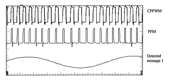
Fig. 5. 35 Recorded waveforms of the first channel demodulation (both modulation are exist, M = 15%,  $\beta = 1$ ,  $f_1 = 130$  kHz,  $f_2 = 50$ kHz).
