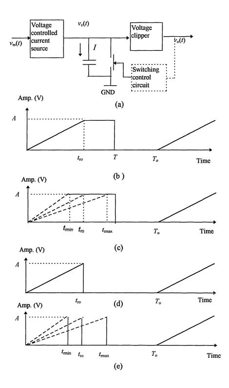
Fig. 3.1 (a) PSM modulator (for triangular PSM control circuit shown dotted is used), (b) trapezoidal PSM waveform in the absence of modulation (c) trapezoidal PSM waveform when modulation is exist (d) triangular PSM waveform in the absence of modulation and (e) triangular PSM when modulation is exist.
