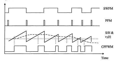
Fig. 5.2 CPFW waveforms when using double edge differentiation.
