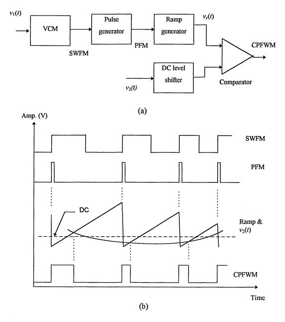
Fig. 5.1 CPFWM modulator: (a) block diagram and (b) waveforms.
