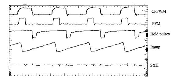
Fig. 5.29 Recorded waveforms at the receiver when both frequency and width modulations are absent ( $\beta = M = 0$ ).
