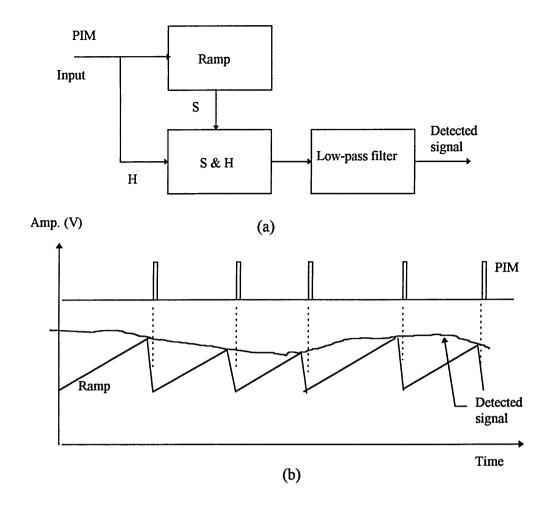
Fig. 2.14 PIM demodulator: (a) block diagram and (b) waveforms.
