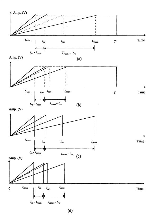
Fig. 3.2 PSM waveform: (a) trapezoidal PSM with high modulation depth, (b) trapezoidal PSM with low modulation depth, (c) triangular PSM with high modulation depth and (d) triangular PSM with low modulation depth.
