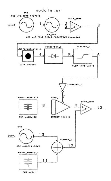
Fig. 5.10 CPFWM modulator block diagram.
