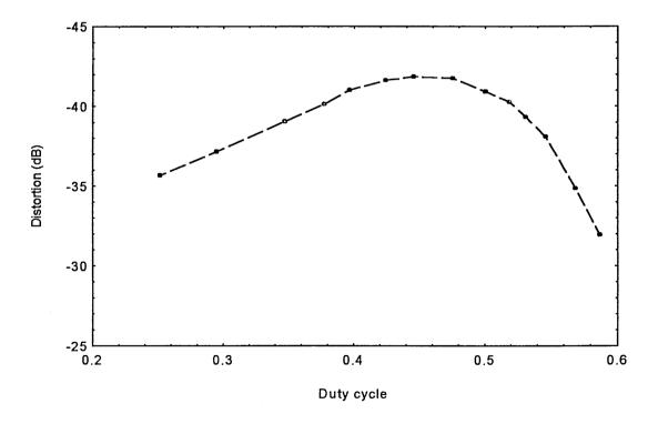
Fig. 5.36 Non-linear distortion in PWM channel as a function of duty cycle,  $f_0 = 1$  MHz,  $f_2 = 100$  kHz, M = 20%.
