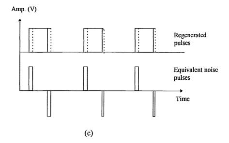
Fig. 7.25 Typical PTM receiver: (a) block diagram, (b) received pulse with noise and (c) time diagram.
