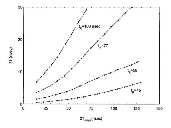
Fig. 7.4 Variation of time jitter with maximum pulse width deviation ( $T_0=500$  nsec).
