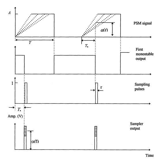
Fig. 3.7 Timing diagram of the proposed PSM demodulator.
