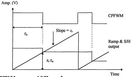
Fig. 5.8 CPFWM, ramp and S/H waveforms.
