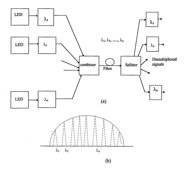
Fig. 4.3 WDM using filtering devices: (a) system block diagram and (b) LED spectrum.
