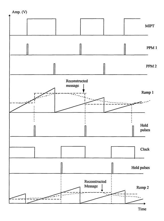
Fig. 4.8 Waveforms of the MIPTM receiver.
