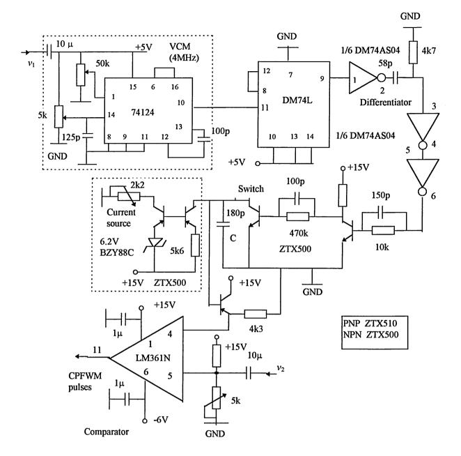
Fig. 5.21 Circuit diagram of the CPFWM modulator.
