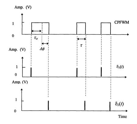
Fig. 6.1 CPFWM and impulse waveform.
