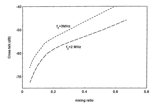
Fig. 4.18 Cross-talk in pulsed FWM system (from second channel to FM ( $f_0 = 21$  MHz,  $\Delta f = 8$  MHz, third order Bessel band pass filter is assumed) [31].
