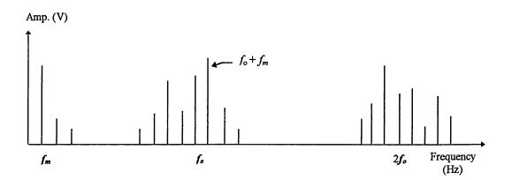
Fig. 2.13 Frequency spectrum for single tone PIM.
