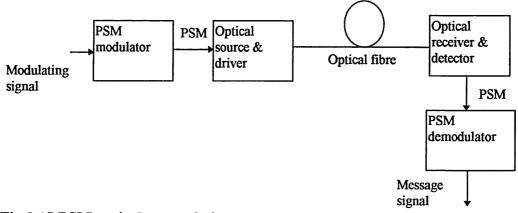
Fig 3.15 PSM optical transmission.
