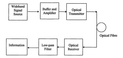
Fig. 2.1 Analogue optical fibre transmission system.
