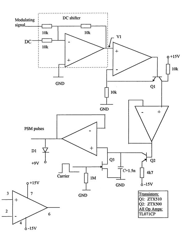
Fig. 3. 20 Circuit diagram of PSM transmitter.
