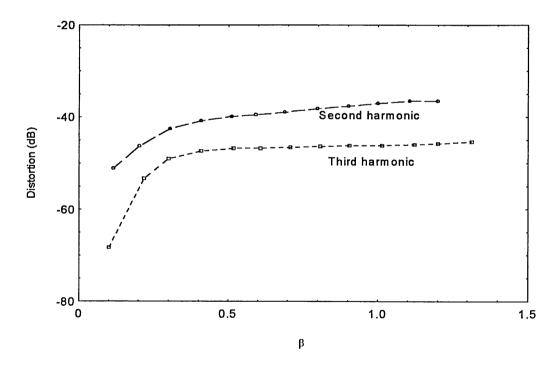
Fig. 5.38 Non-linear distortion in PFM channel,  $f_0 = 1$  MHz,  $f_1 = 120$  kHz and 50% Duty cycle.
