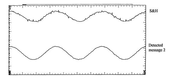
Fig. 5. 33 Recorded waveforms of the second detected message (M = 15%,  $\beta = 1$ ,  $f_1 = 130$  kHz,  $f_2 = 50$ kHz).
