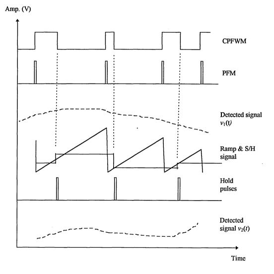
Fig. 5.7 Waveforms of the CPFWM demodulator.
