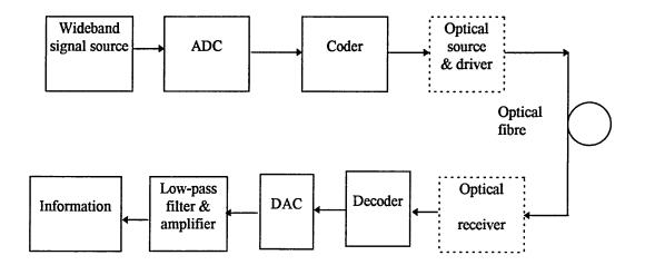
Fig. 2.3 Typical digital transmission system block diagram.
