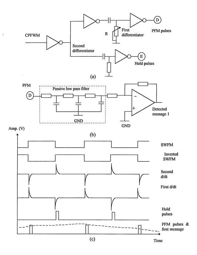
Fig. 5.19 Edge separation and PFM demodulation: (a) edge separation circuit diagram, (b) PFM demodulator and (c) waveforms.
