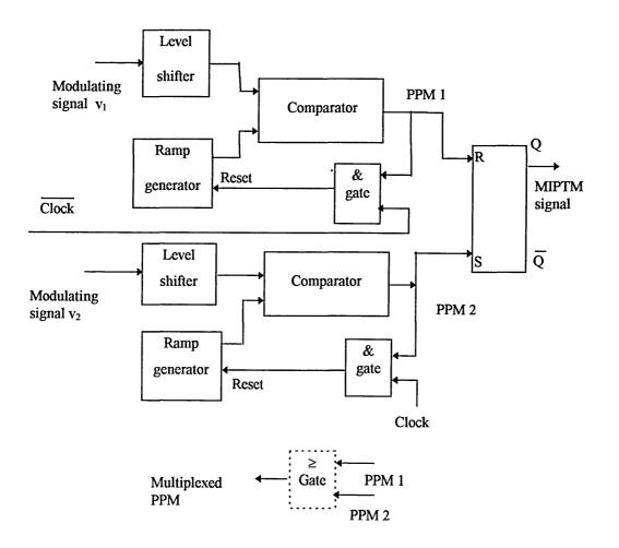
Fig. 4.5 Block diagram of MIPTM system.
