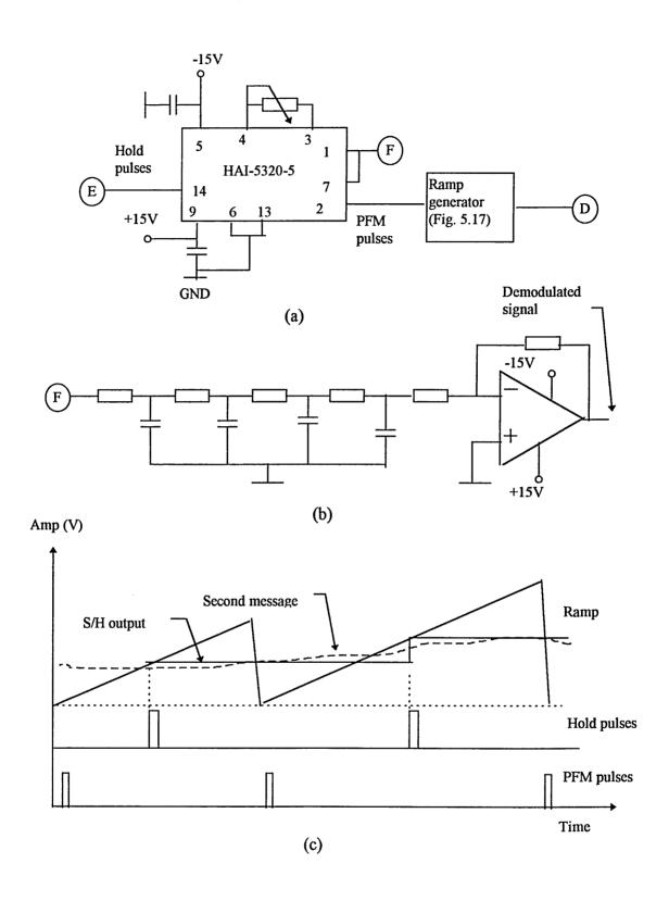
Fig 5.20 Detection of the second modulating signal: (a) sample and hold amplifier, (b) output filter and (c) waveforms.
