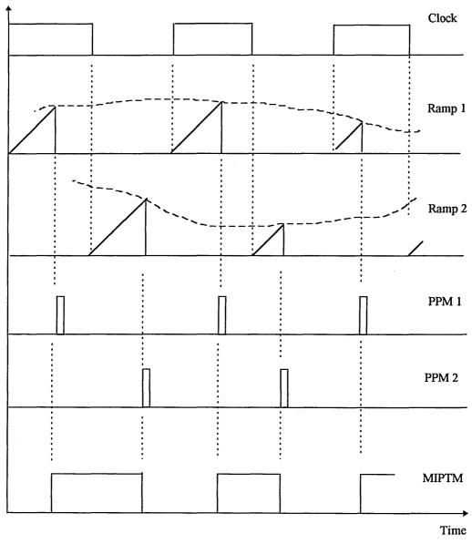
Fig. 4.6 MIPTM multiplexing waveforms.
