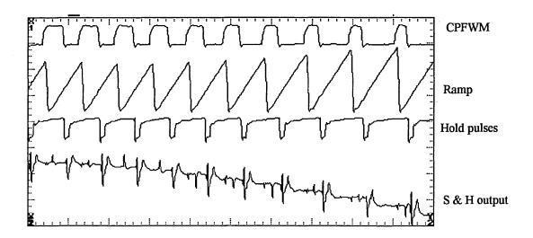
Fig. 5. 34 Recorded waveforms of the second channel demodulation (both modulation are exist, M = 15%,  $\beta = 1$ ,  $f_1 = 130$  kHz,  $f_2 = 50$ kHz).
