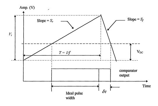
Fig. 5.5 Comparator output and ramp waveforms.
