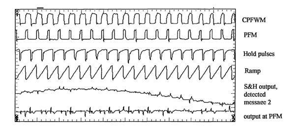
Fig 5. 31 Recorded waveforms at the receiver when frequency modulation is absent ( $\beta = 0$ ), and, M = 15%,  $f_2 = 50$  kHz.
