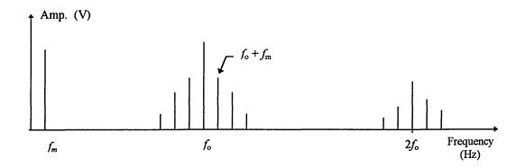
Fig. 2.8 Frequency spectrum for single tone PWM waveform (naturally sampled).
