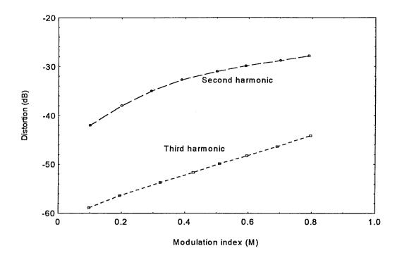
Fig. 5.37 Non-linear distortion in PWM channel,  $f_0 = 1$  MHz,  $f_2 = 100$  kHz and
