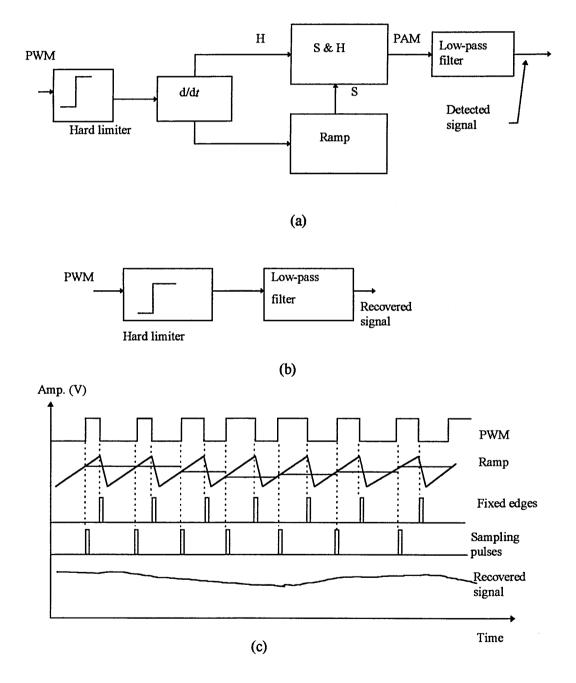
Fig. 2.9 PWM demodulator: (a) uniformly sampled, (b) naturally sampled and (c) waveforms.
