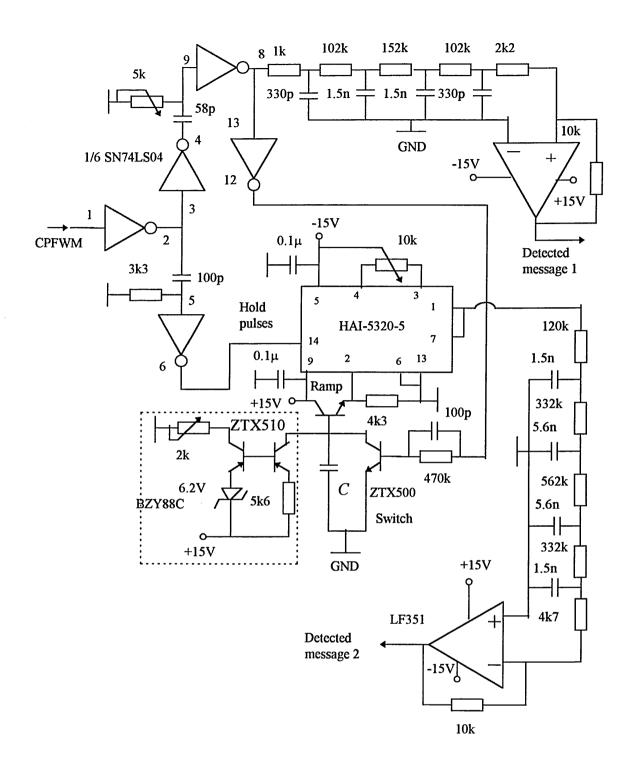
Fig. 5.22 Circuit diagram of the CPFWM demodulator.
