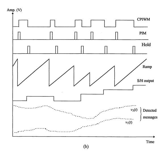
Fig. 4.12 CPIWM receiver: (a) block diagram and (b) waveforms.
