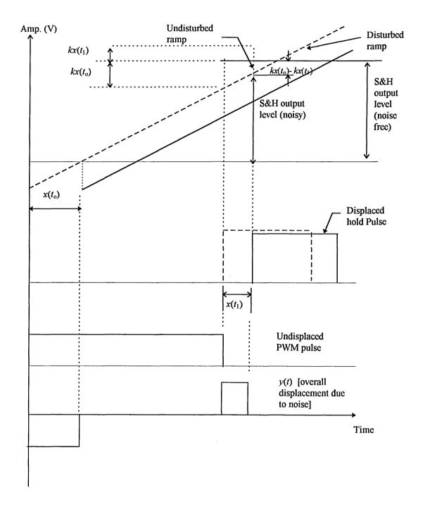
Fig. 7.31 Regenerated signal at the sample and hold amplifier when noise is present.
