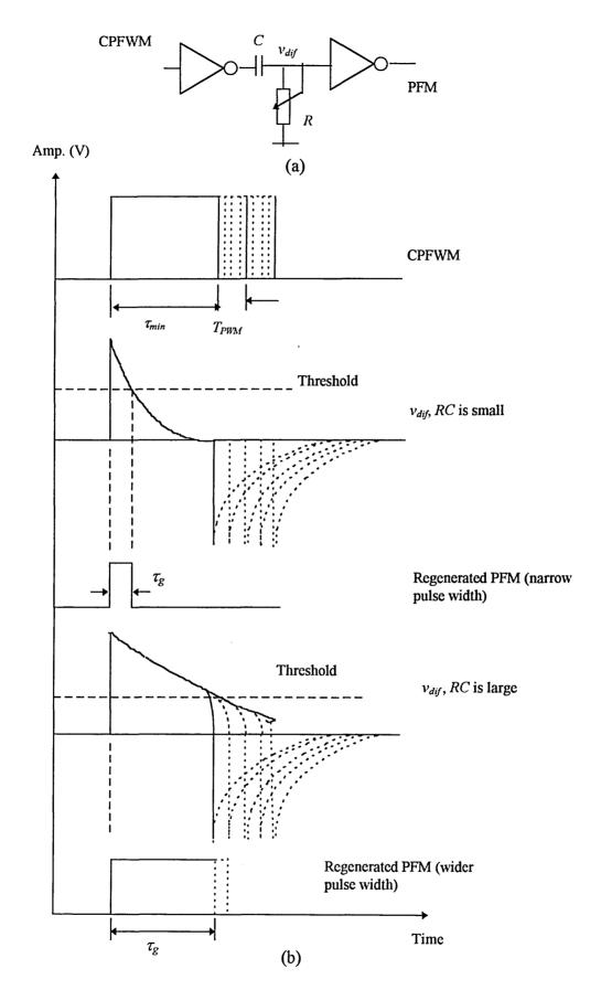
Fig. 7.11 Edge separation at the CPFWM receiver: (a) circuit diagram and (b) waveforms.
