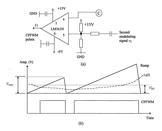
Fig. 5.18 Comparator: (a) circuit diagram and (b) waveforms.
