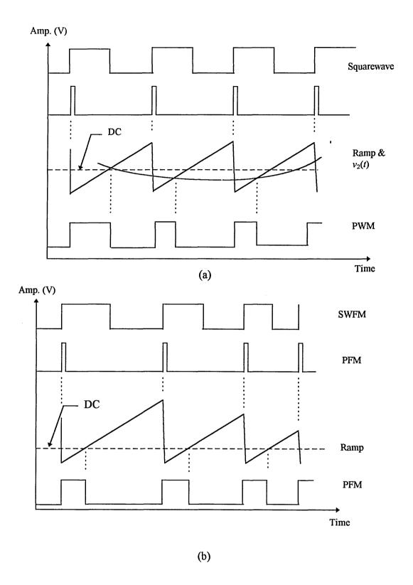
Fig. 5.3 Waveforms of the CPFWM modulator: (a) when the first input is removed and (b) when the second input is removed.
