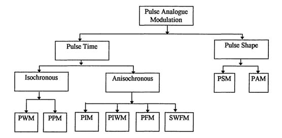
Fig. 2.6 Pulse analogue modulation tree.
