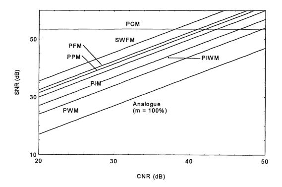
Fig. 2.29 Theoretical noise performance of different modulation schemes.
