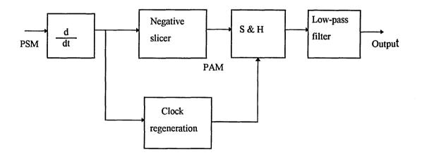
Fig. 3.5 PSM demodulator using sample and hold.
