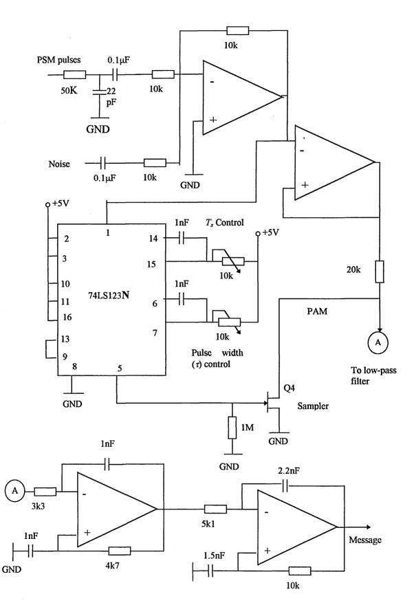
Fig. 3.21 Circuit diagram of PSM receiver (all op. amps are TL071CP).
