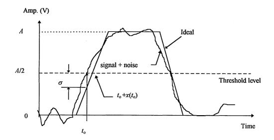
Fig. 2.26 General PTM waveform with noise.
