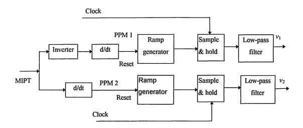
Fig. 4.7 Block diagram of MIPTM receiver.
