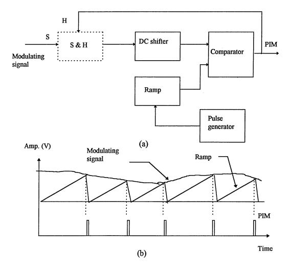
Fig 2.12 PIM modulator: (a) block diagram and (b) waveforms.
