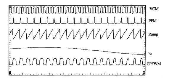
Fig. 5. 27 Recorded waveforms at the CPFWM, when M = 15% and  $f_2 = 50$  kHz, and frequency modulation is absent ( $\beta = 0$ ).
