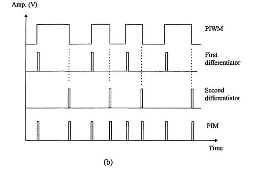
Fig. 2.17 PIWM to PIM converter (a) circuit diagram and (b) waveforms.
