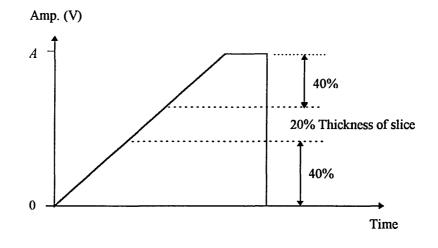
Fig. 3.16 Slicing level of the PSM signal.
