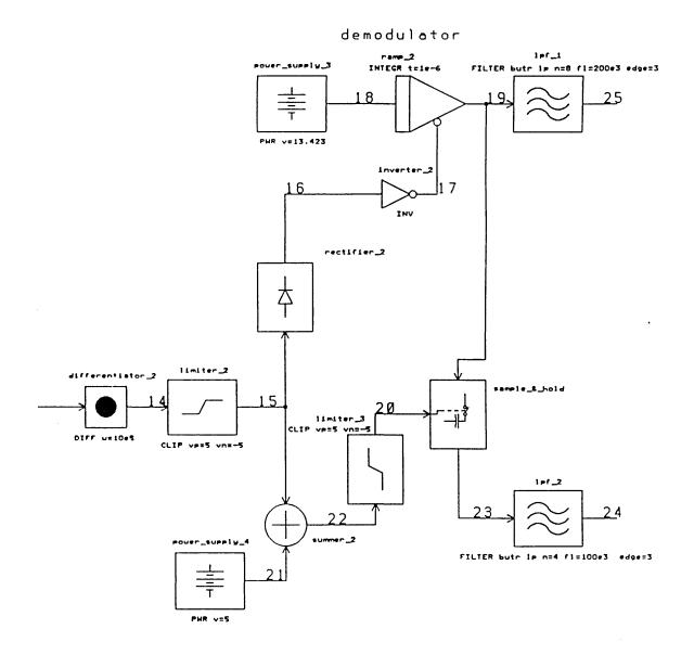
Fig. 5.12 Simulator block diagram of CPFWM demodulator.
