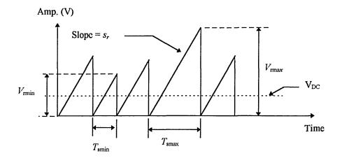
Fig. 5.4 Waveforms at the comparator inputs.
