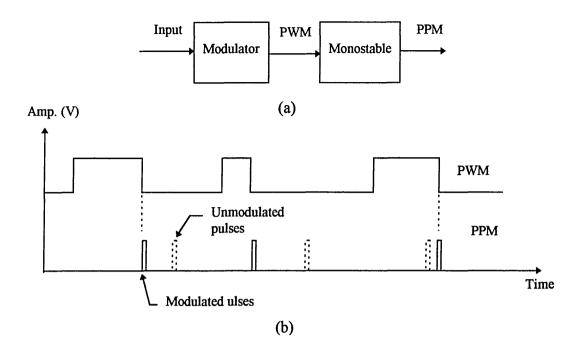
Fig. 2.10 PPM modulator: (a) block diagram and (b) waveforms.
