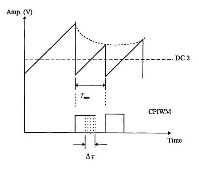
Fig. 4.11 Modulated ramp waveform and CPIWM signal.
