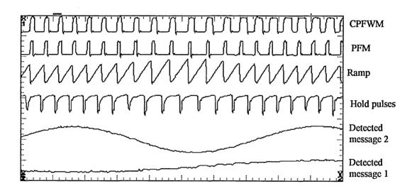
Fig 5. 32 Recorded waveforms at the receiver when both width frequency modulation and are exist, ( $\beta = 1$ , M = 15%,  $f_1 = 130$  kHz, and  $f_2 = 60$  kHz).
