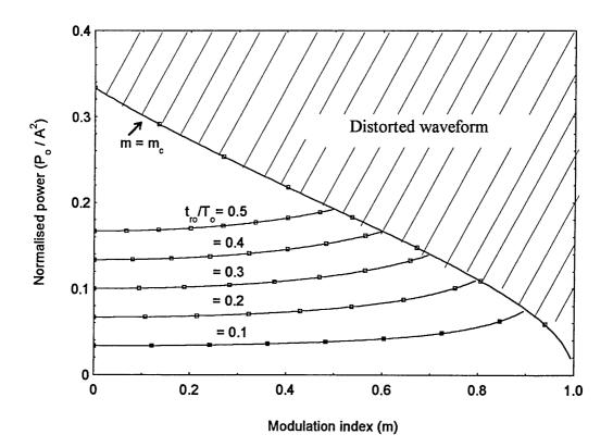
Fig. 3.12 Normalised average power for triangular PSM waveforms.
