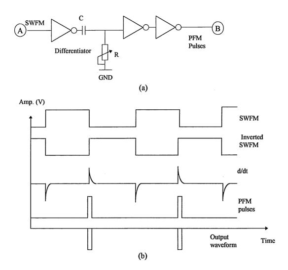
Fig. 5.16 SWFM pulses differentiation: (a) circuit diagram and (b) waveforms.
