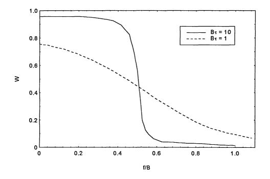
Fig. 3.19 Normalised noise power spectral density of PSM system.
