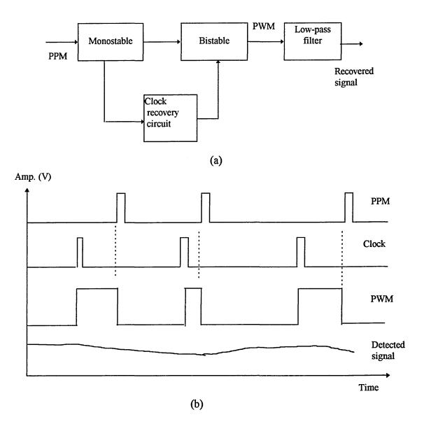
Fig. 2.11 PPM demodulator: (a) block diagram and (b) waveforms.
