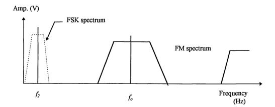
Fig. 4.16 Frequency spectrum of pulsed FWM waveform.
