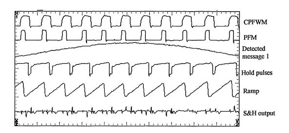
Fig 5. 30 Recorded waveforms at the receiver when width modulation is absent (M = 0), and  $\beta = 1$ ,  $f_1 = 130$ kHz.
