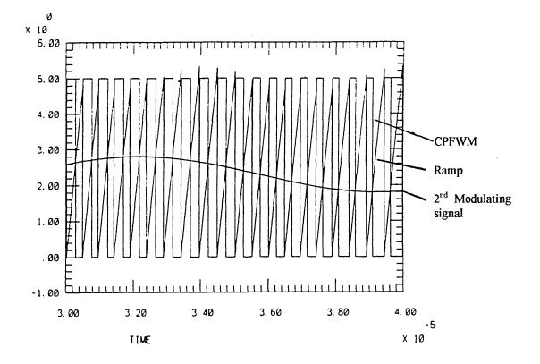
Fig. 5.11 Waveforms of the simulated CPFWM modulator.
