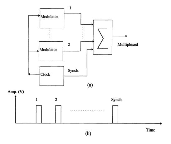
Fig. 4.1 Synchronous TDM: (a) possible block diagram and (b) timing diagram.
