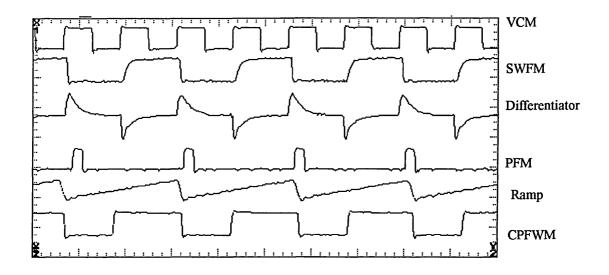
Fig. 5.25 Recorded waveforms at the CPFWM transmitter, when both modulating signals are absent (i.e.  $M = \beta = 0$ )
