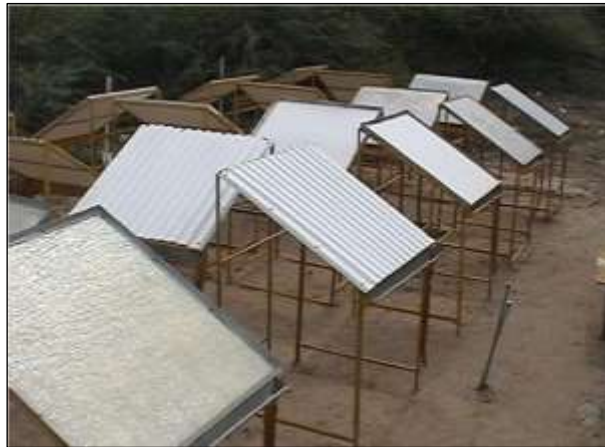
Figure 3: Different types of condenser surfaces investigated (Sharan, 2011).
