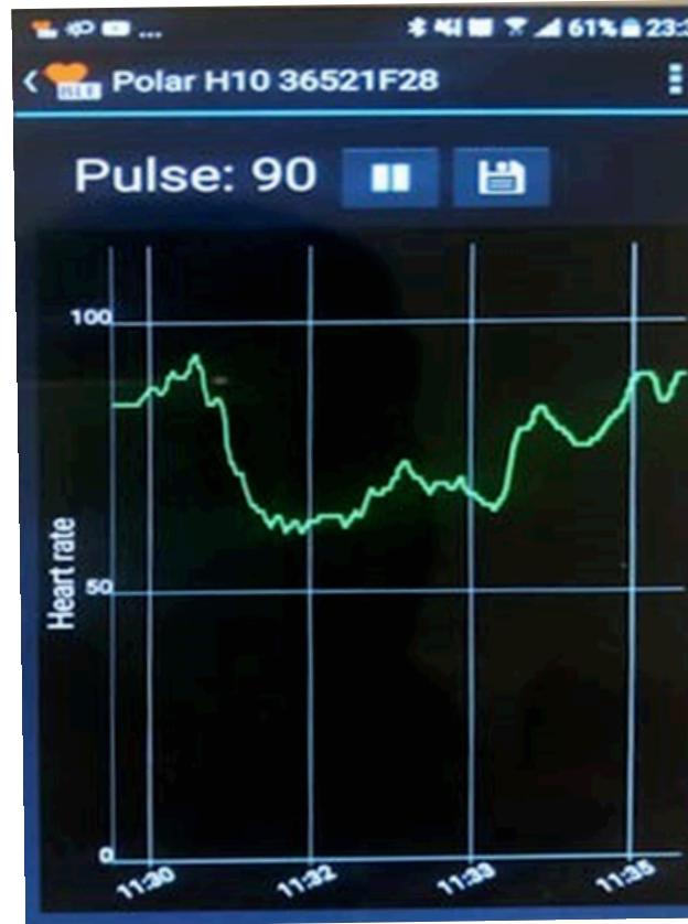
Figure 6. HR signals appear on the smartphone screen.
