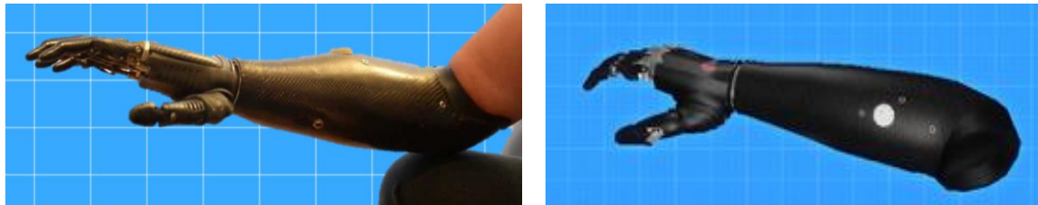
Figure 2: To the right, the real Bebionic prosthetic arm. To the left, the VR Bebionic 3D model of the prosthetic arm.
